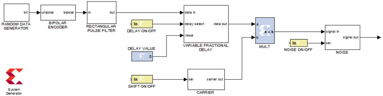
Fig. 5. Top-level circuit of the BPSK signal generator in the System Generator environment.
