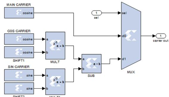
Fig. 8. The Carrier block with selectable phase and frequency shifts.
