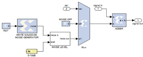
Fig. 9. The circuit that implements the Noise block. SNR and the presence of noise are selectable within this block.
