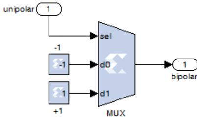
Fig. 6. The Bipolar Encoder block expanded. A multiplexer and two constants compose the encoder.
