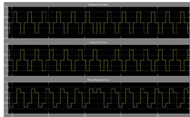
Fig. 11. Time-domain analysis of the discrete BPSK signal. Reference waveform (top). Delayed version of reference waveform (middle). Reference waveform with phase and frequency errors (bottom).
