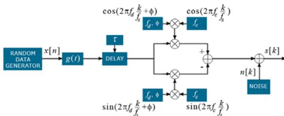
Fig. 2. Block diagram of the circuit that generates the discrete BPSK signal,  $s[k]$ .
