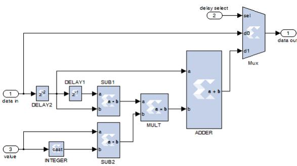
Fig. 7. Detailed implementation of the Variable Fractional Delay block. Adders, multipliers, subtraction and delay blocks perform linear interpolation of the input signal.
