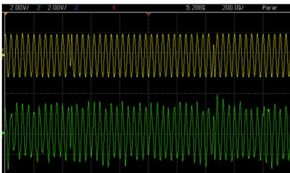
Fig. 14. Time-domain analysis of the BPSK signal with an oscilloscope. Reference waveform (top) showing two symbol transitions. (Bottom) Reference waveform with added Gaussian noise (SNR = 8dB).
