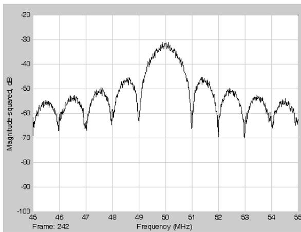
Fig. 12. Spectrum analysis of the BPSK signal in the System Generator environment.
