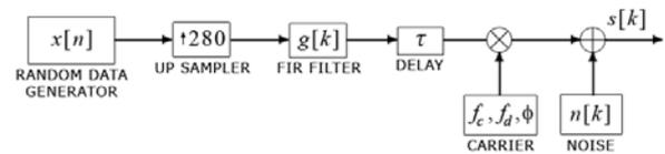
Fig. 3. High-level diagram of the BPSK signal generator in the Simulink environment.
