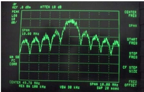
Fig. 13. Spectrum analysis of the BPSK signal in a Spectrum Analyzer.
