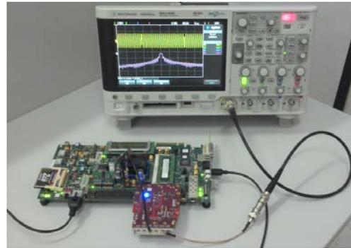
Fig. 10. Test bench showing the BPSK signal generator running in FPGA. The oscilloscope screen shows the input signal both in the time (top) and frequency (bottom) domains.
