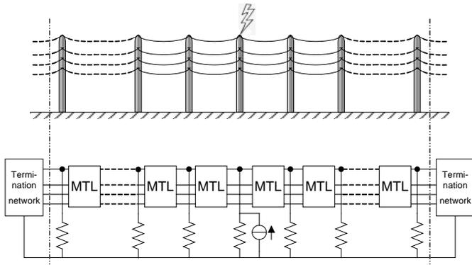
Fig. 6 Configuration considered (top) and equivalent circuit (down).
