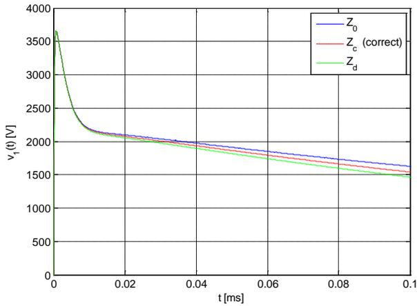
Fig. 9 Voltage  $v_I(t)$  at the hit point.  $R_g = 1 \Omega$ ,  $\ell = 300$  m.
