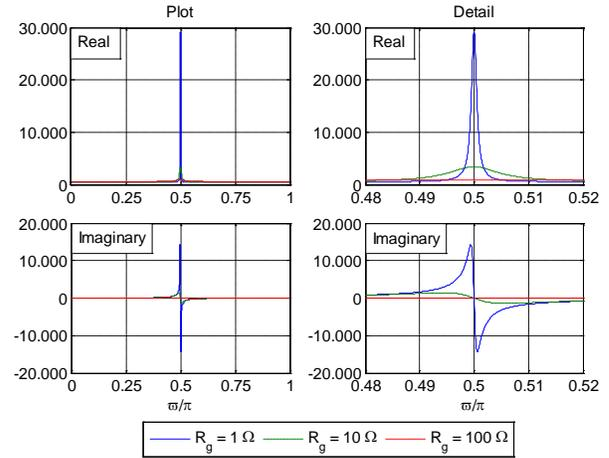
Fig. 5 Coefficient  $\dot{Z}_{c,(11)}$ : plot over an entire period (left hand side) and zoom in (right hand side). Distance  $\ell = 300 \text{ m}$ .
