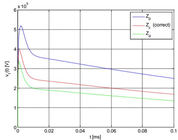
Fig. 8 Voltage  $v_1(t)$  at the hit point.  $R_g = 100 \Omega$ ,  $\ell = 50$  m.
