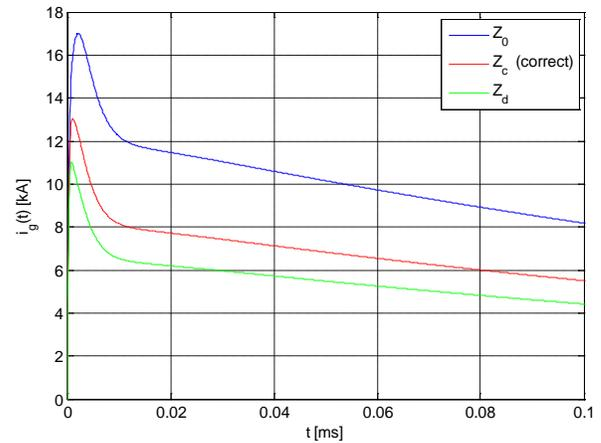
Fig. 11 Current  $i_g(t)$  flowing through the grounding at the hit point.  $R_g = 100 \Omega$ ,  $\ell = 50$  m.
