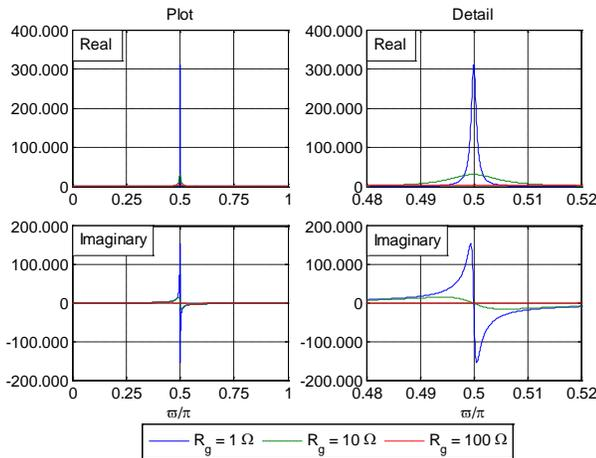
Fig. 4 Coefficient  $\dot{Z}_{c,(7,7)}$ : plot over an entire period (left hand side) and zoom in (right hand side). Distance  $\ell = 50 \text{ m}$ .
