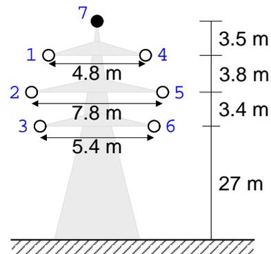
Fig. 2 Line geometry: conductors 1-6 are phase conductors, conductor 7 is the periodically grounded shield wire.
