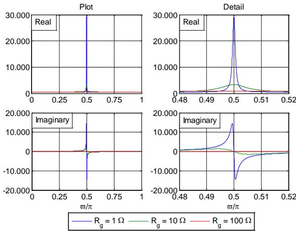
Fig. 3 Coefficient  $\dot{Z}_{c,(11)}$ : plot over an entire period (left hand side) and zoom in (right hand side). Distance  $\ell = 50 \text{ m}$ .
