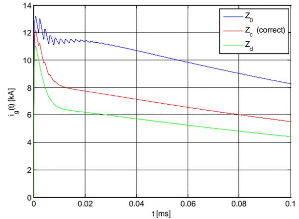
Fig. 12 Current  $i_g(t)$  flowing through the grounding at the hit point.  $R_g = 100 \Omega$ ,  $\ell = 300$  m.
