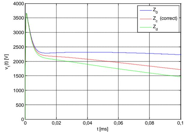
Fig. 7 Voltage  $v_1(t)$  at the hit point.  $R_g = 1 \Omega$ ,  $\ell = 50$  m.
