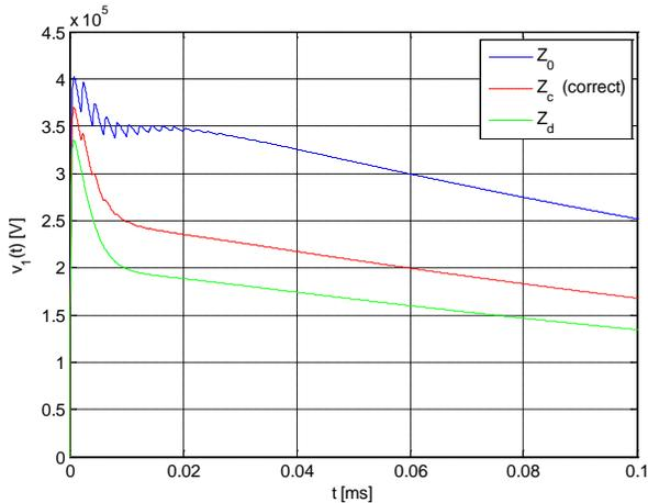
Fig. 10 Voltage  $v_I(t)$  at the hit point.  $R_g = 100 \Omega$ ,  $\ell = 300$  m.
