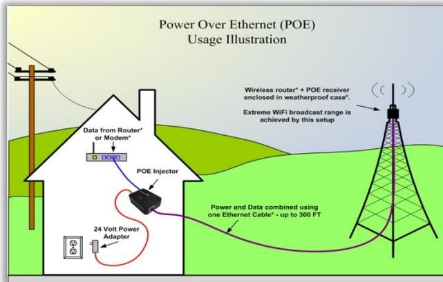
Fig 2. PoE device installed outdoors [8]
