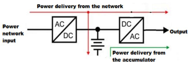
Fig. 4 On-line UPS block diagram [2]
