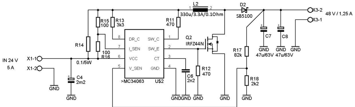
Fig. 15 Connection diagram of Step-up converter with MC34063
