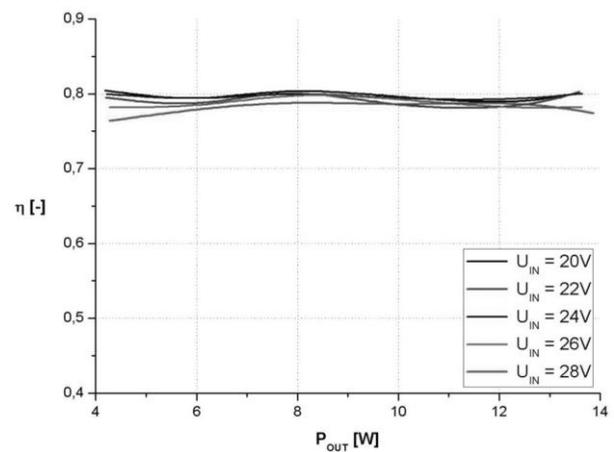
Fig. 13 Power efficiency of the converter vs. output power
