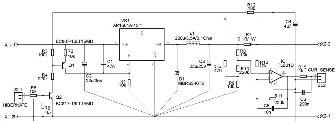
Fig. 11 Connection diagram of Step-down converter with AP1501A-12
