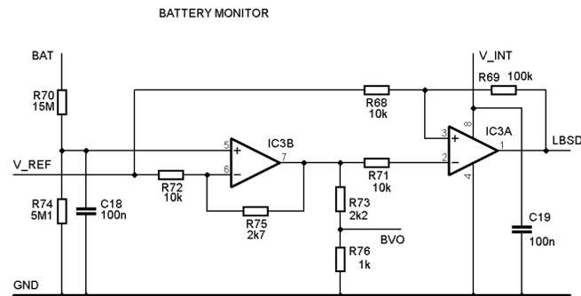
Fig. 10 Connection diagram of the Battery monitor
