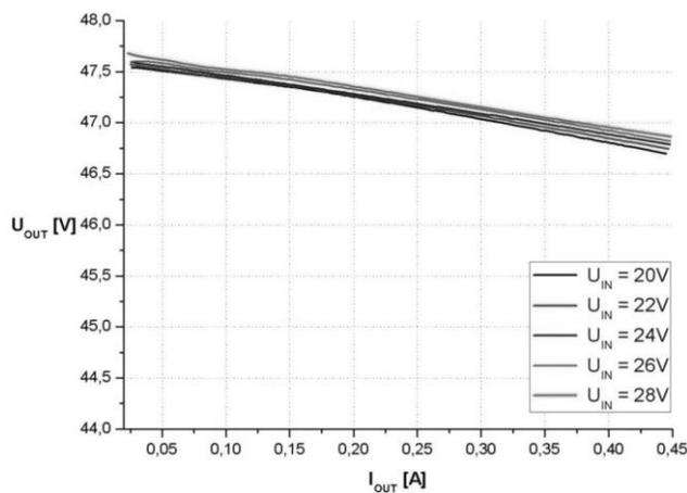
Fig. 18 Output voltage of the converter vs. output current
