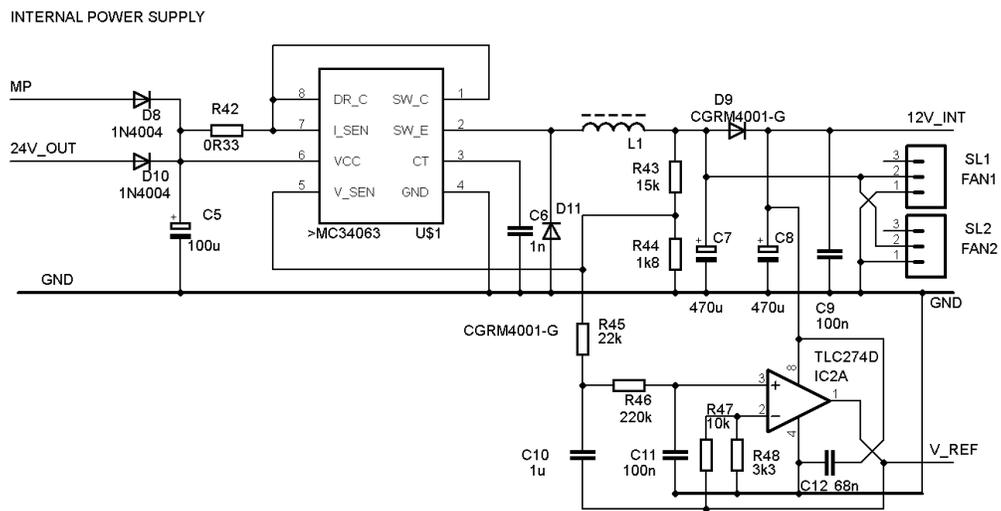
Fig. 7 Connection diagram of Internal power supply block
