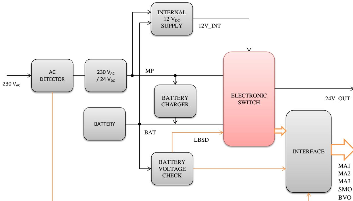
Fig.5 Electronic switch block diagram
