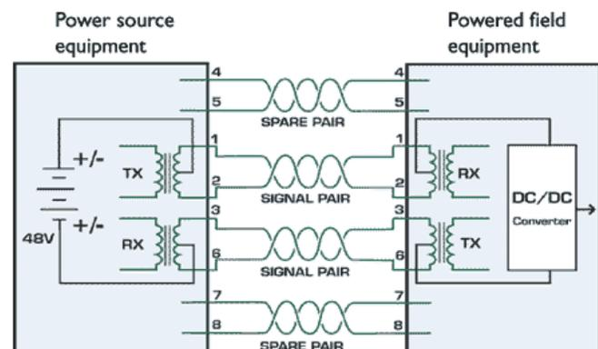
Fig. 1 Power over Ethernet principle [7]
