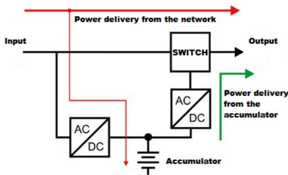
Fig. 3 Off-line UPS block diagram [2]
