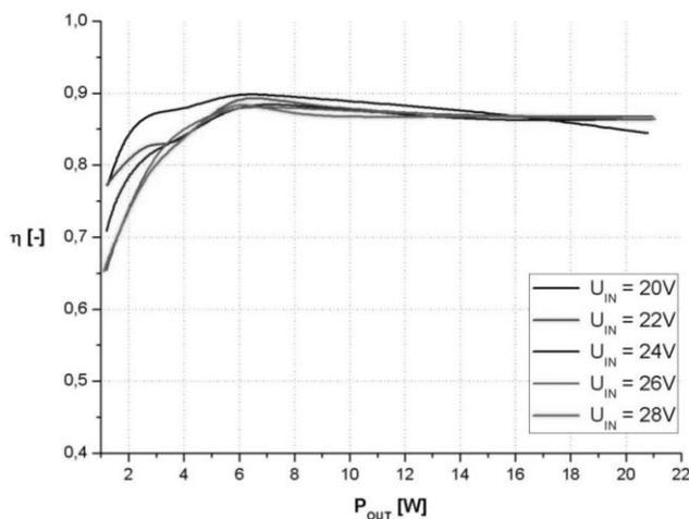
Fig. 19 Power efficiency of the converter vs. output power
