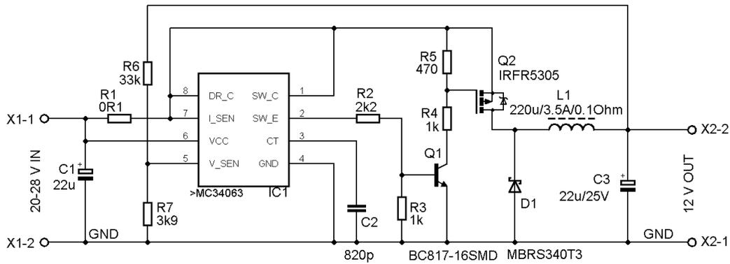
Fig. 14 Connection diagram of Step-down converter with MC34063
