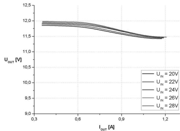
Fig. 12 Output voltage of the converter vs. output current
