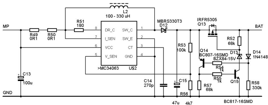
Fig. 8 Connection diagram of Battery charger
