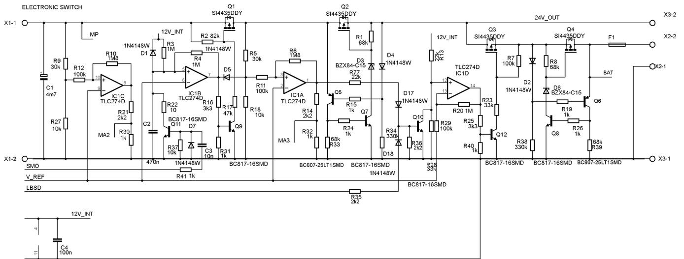
Fig. 6 Connection diagram of the Electronic switch
