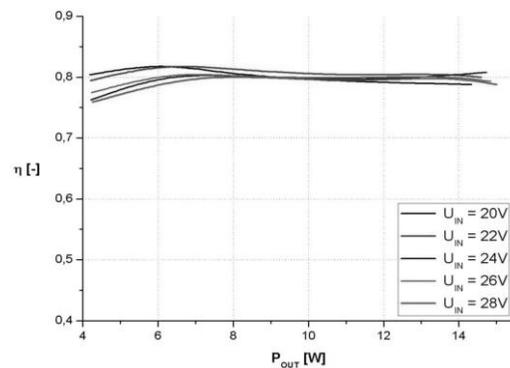
Fig. 17 Power efficiency of the converter vs. output power
