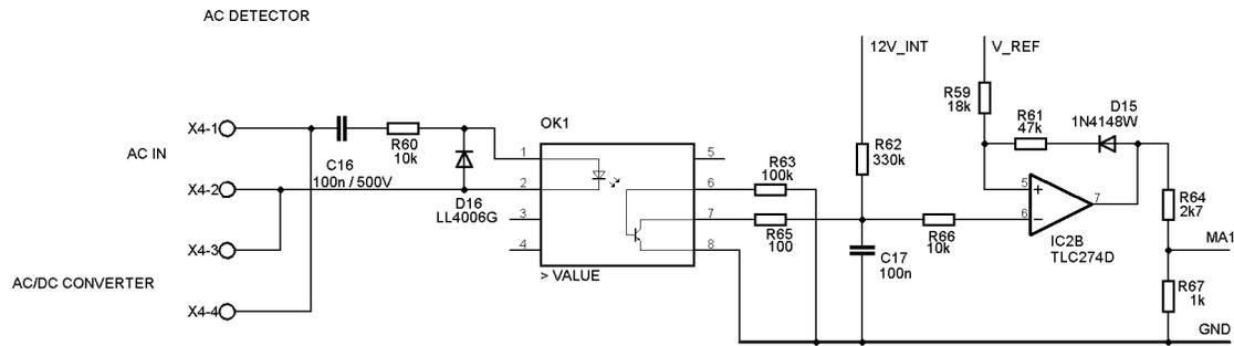
Fig. 9 Connection diagram of the AC detector circuit
