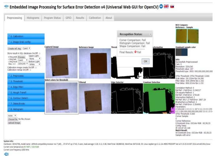
Fig. 21 Image processing GUI (Raspberry PI).
