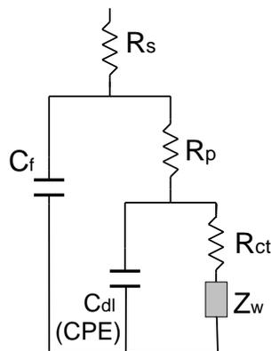
Fig. 4 - Equivalent circuit utilized for fitting the EIS spectra
