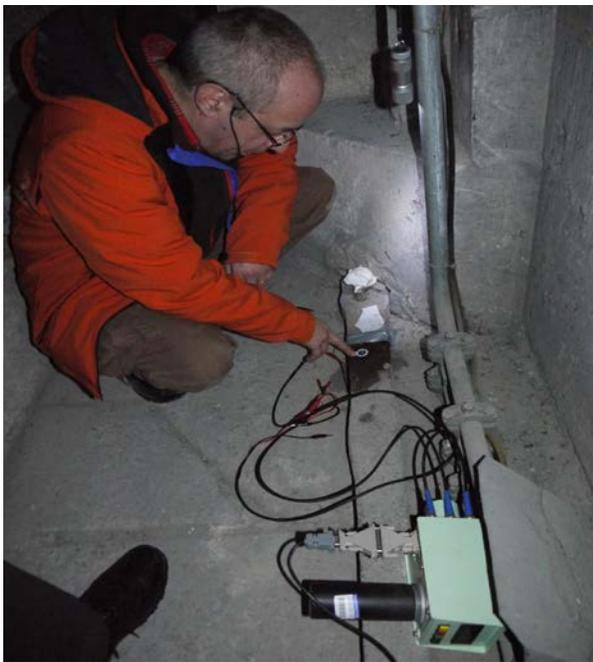
Fig. 2 - In situ EIS measurements monitoring campaign on the iron bar chain of the Notre-Dame Cathedral with the portable instrumentation.
