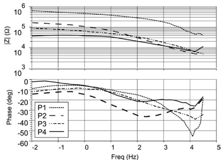
Fig. 3 - Bode plots (impedance modulus,  $|Z|$ , and phase) recorded onto different areas of the iron bar chain of the Notre-Dame Cathedral and the structural phase contents of the analysed areas.
