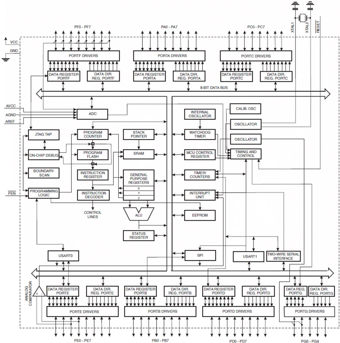
Fig. 1 Block Diagram of the AVR Architecture [5]
