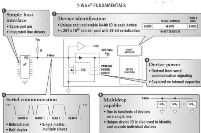
Fig. 10 1-Wire Bus basic circuit [19]
