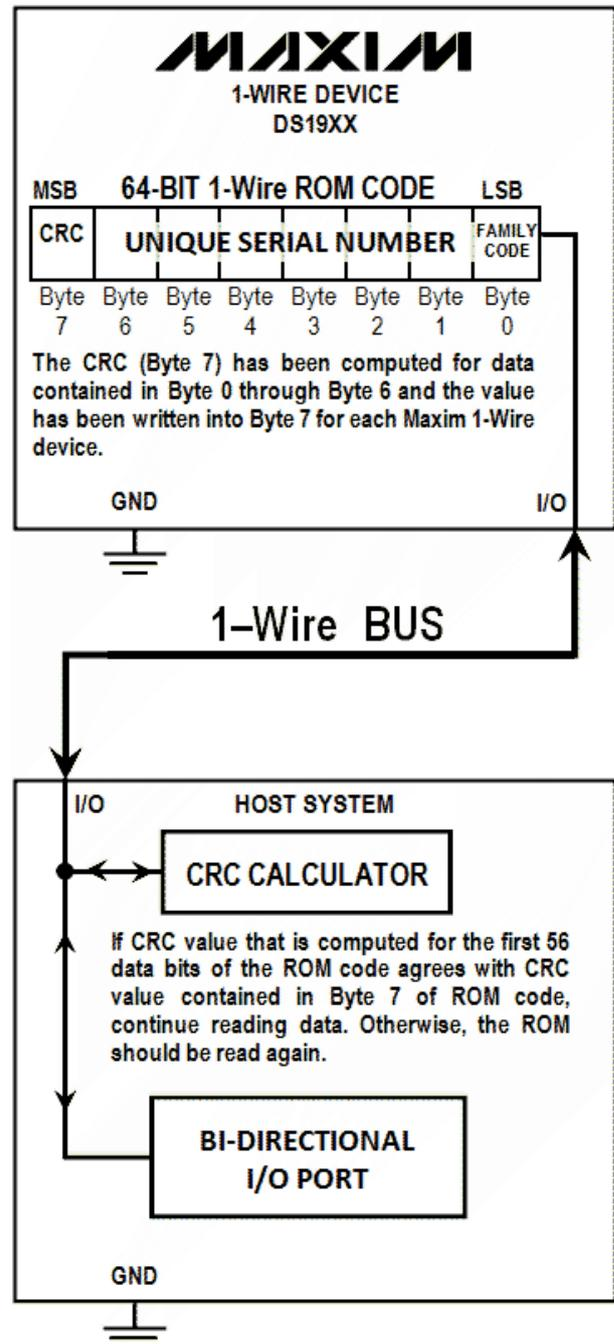
Fig. 9 The iButton checksum read up [18]
