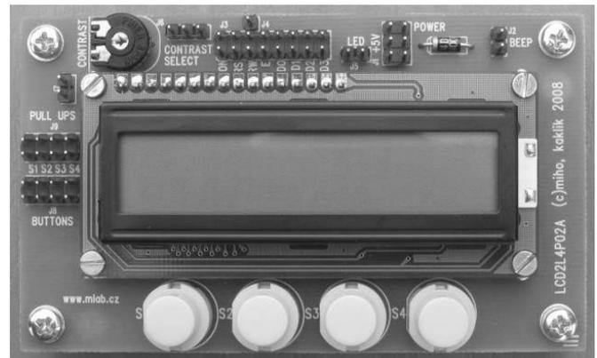
Fig. 4 LCD module with control buttons [17]
