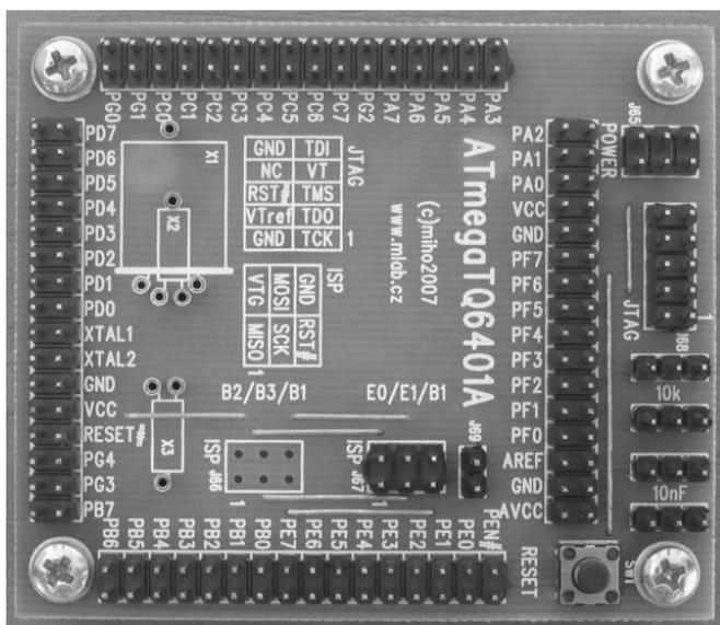
Fig. 3 ATmega128 MCU module [16]
