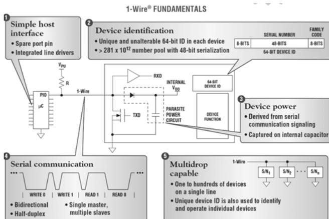
Fig. 10 1-Wire Bus basic circuit [19]
