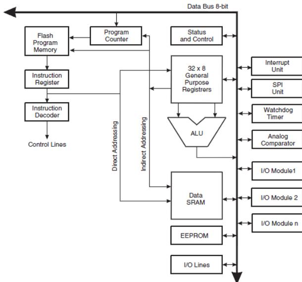
Fig. 2 Block Diagram of the AVR Architecture [5]
