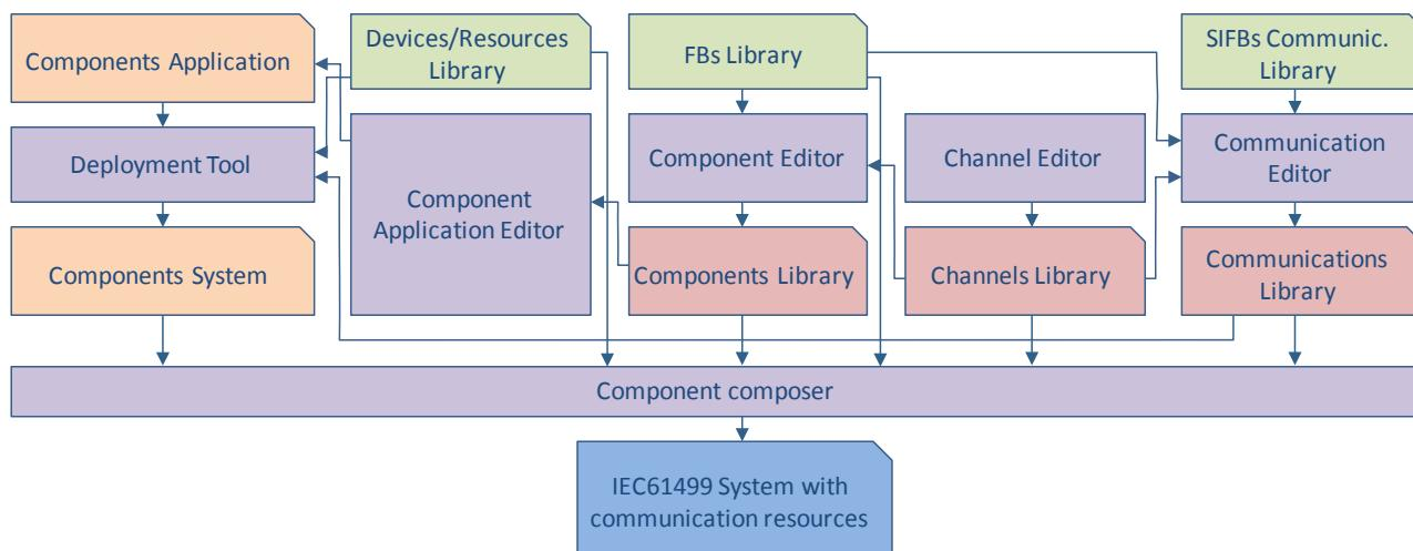
Fig. 7. IEC 61499 system development with components, translate and composition.
