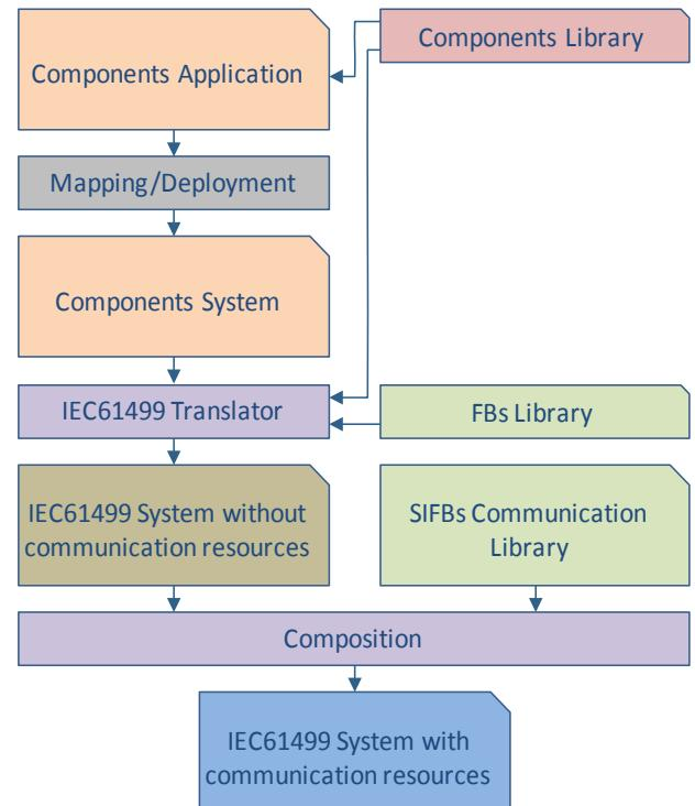
Fig. 6. IEC 61499 system development with components, translate and composition.
