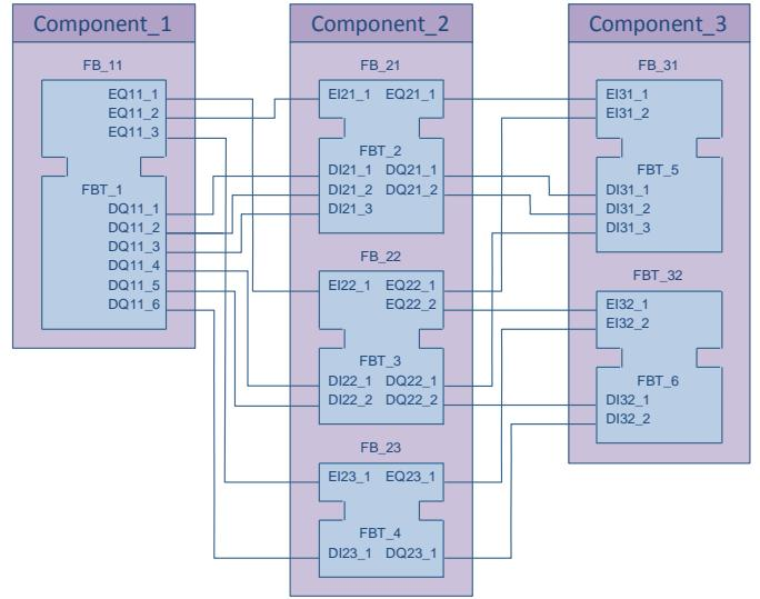
Fig. 1. FB-based programming to automation components.
