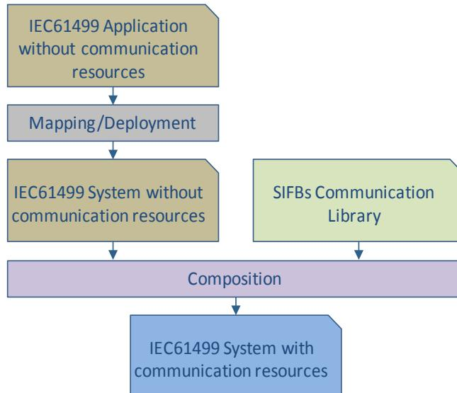
Fig. 5. IEC 61499 system development with composition.
