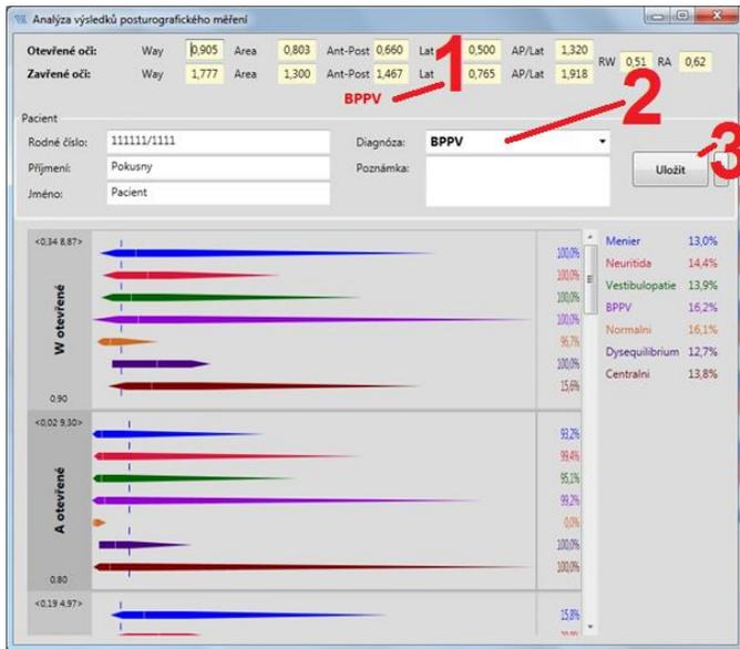
Fig. 14 Software “Analysis of the results of posturography measurement” – program description
