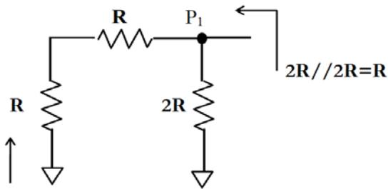
Fig.2: Diagram of a resistor ladder
