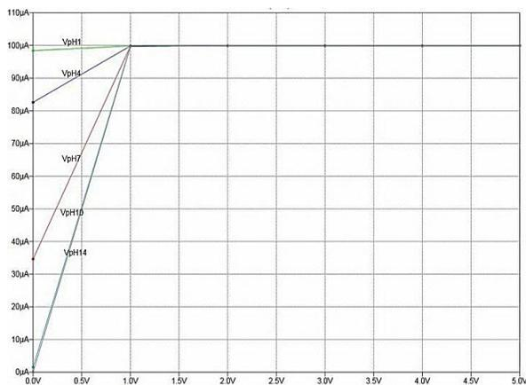
Figure 11: Variation in drain current ( $I_d$ ) with reference voltage ( $V_{ref}$ )
