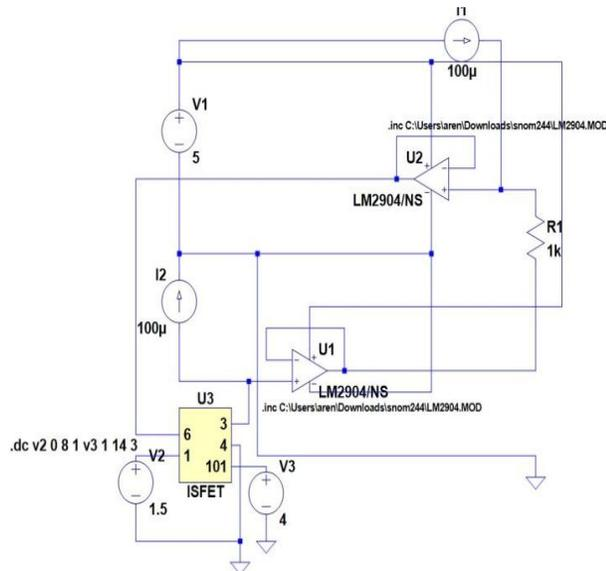
Figure 5: Schematic Diagram of ISFET Macromodel Readout Circuit
