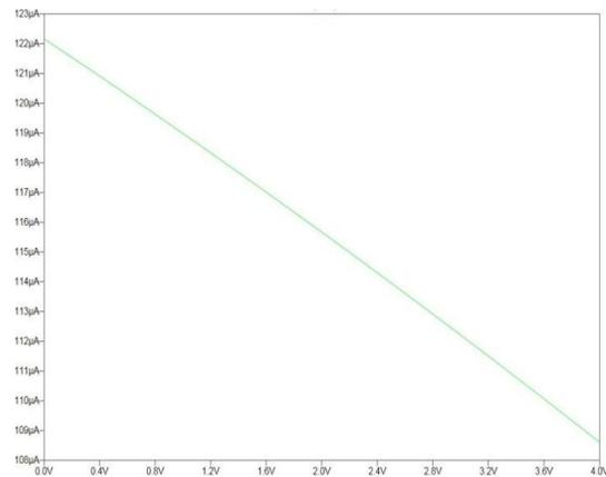
Figure 7: Variation in drain current ( $I_d$ ) with equivalent voltage of pH ( $V_{pH}$ ) at a constant  $V_{ref}$  of 1.5V
