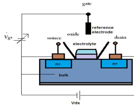
Figure 1: Structure of an ISFET
