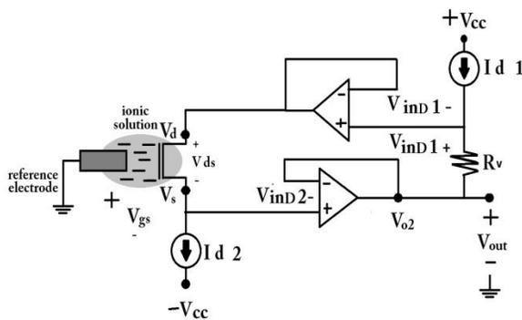
Figure 3: The CVCC readout circuit
