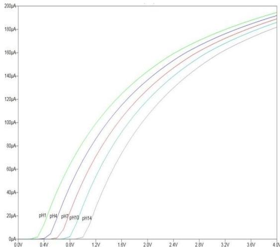
Figure 6: Variation in drain current ( $I_d$ ) with reference voltage ( $V_{ref}$ ) with drain voltage ( $V_d$ ) constant at 0.1V
