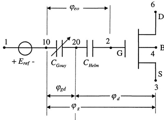
Figure 2: Equivalent circuit of an ISFET
