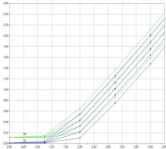
Figure 9: Variation in drain voltage ( $V_d$ ) and source voltage ( $V_s$ ) with reference voltage ( $V_{ref}$ )
