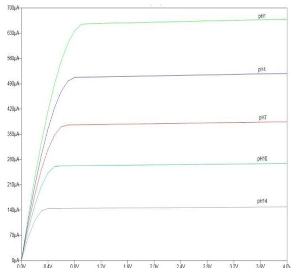
Figure 8: Variation of drain current ( $I_d$ ) with drain voltage ( $V_d$ ) at reference voltage ( $V_{ref}$ ) constant at 1.5V
