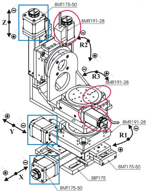
Fig. 8 Construction of positioner
