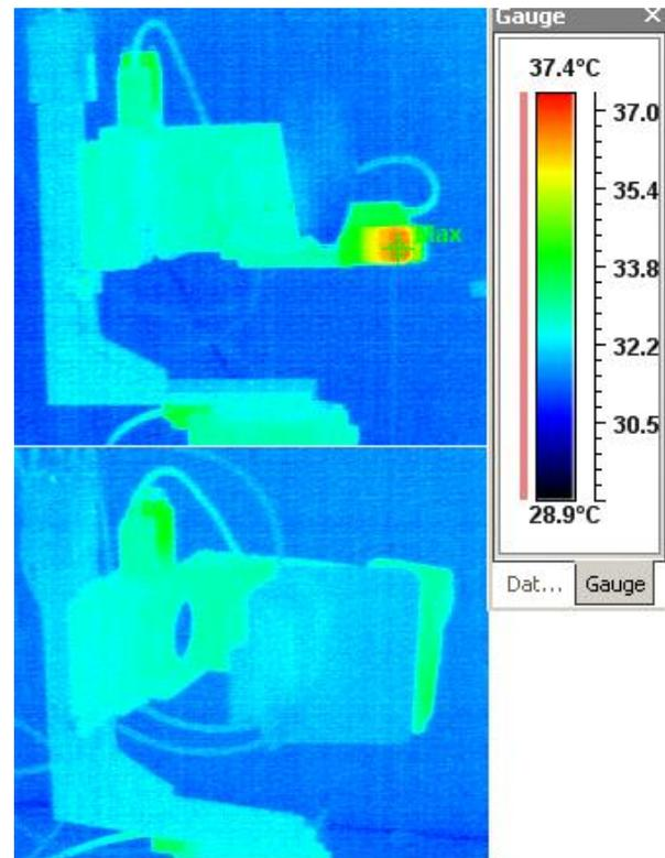
Fig. 12 Comparison of temperatures drive without shielding and with shielding
