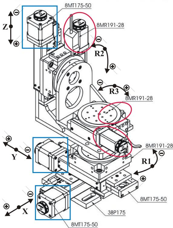
Fig. 8 Construction of positioner
