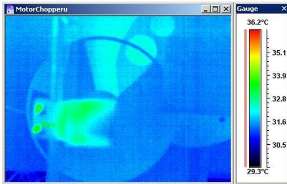
Fig. 5 IR image of the chopper drive
