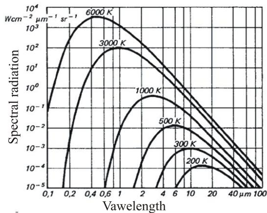
Fig. 3 Blackbody radiation characteristics depending on its temperature
