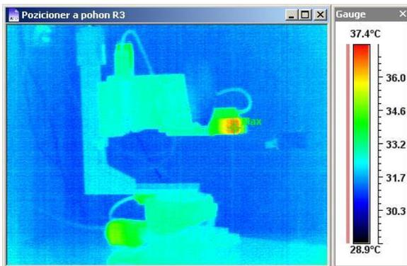
Fig. 6 IR image of the chopper drive
