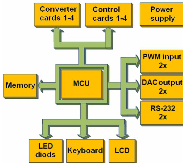
Fig. 4 New laboratory unit functional block scheme
