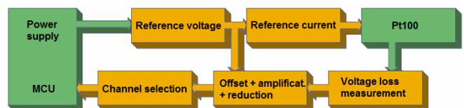
Fig. 8 Converter board functional block scheme
