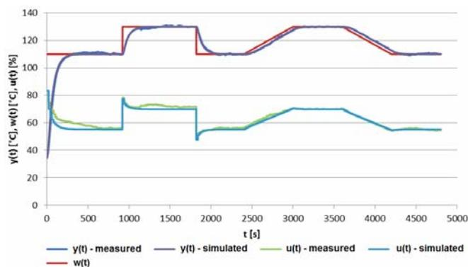
Fig. 18 Control responses for plant (3) with controller (5)
