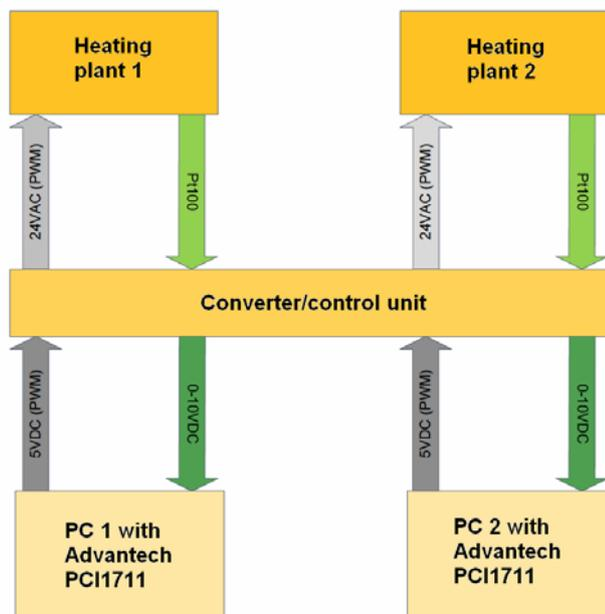
Fig. 1 Laboratory heating system scheme
