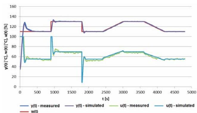
Fig. 19 Control responses for plant (3) with controller (7)
