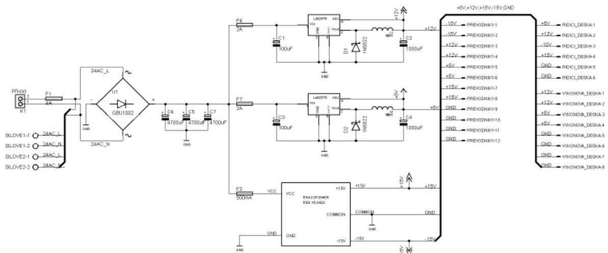
Fig. 12 Power supply electronic circuit scheme
