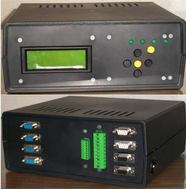
Fig. 13 A photo of the designed I/O converter and control unit – the front (up) and the back side (down)
