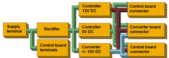
Fig. 11 Power supply functional block scheme
