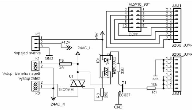
Fig. 10 Control board electronic circuit scheme
