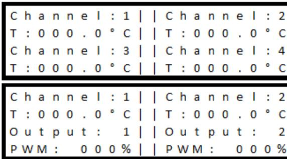
Fig. 16 Display layout for four (up) and two (down) plugged cards
