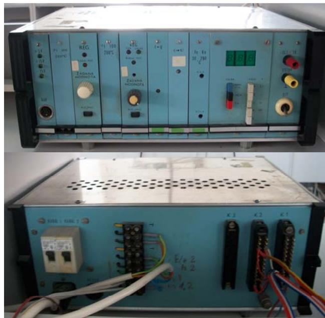
Fig. 2 A photo of the current I/O converter and control unit – the front (up) and the back side (down)
