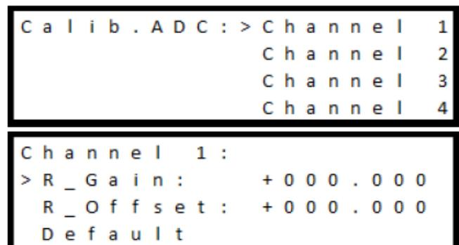
Fig. 17 Display of AD converted signal calibration
