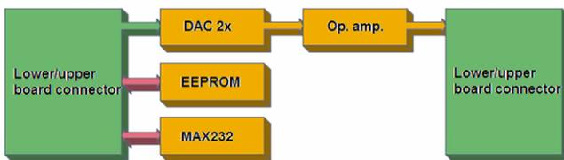
Fig. 6 Lower central board functional block scheme
