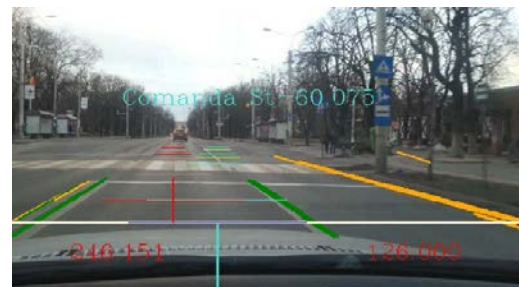
Figure.12 Generated future position of the vehicle based on road lane middle
