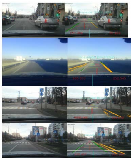
Figure.16 Frames with virtual lanes generated
