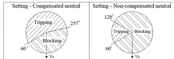
Fig. 8. Calibration of a directional protection.
