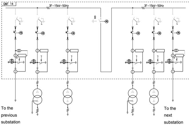
Fig. 3. Details of two secondary, consecutive MV/LV substations from the diagram in Fig.1.
