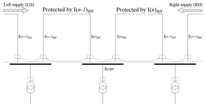
Fig. 4. System layout with the protection mechanism.
