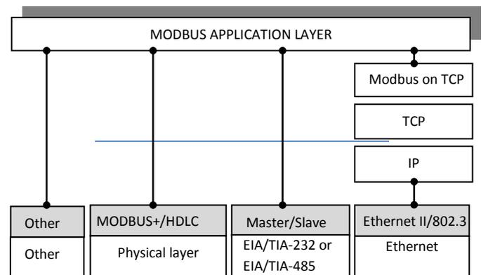
Fig. 11. Modbus communication stack.
