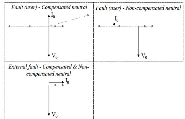
Fig. 7. Conditions for a ground fault, electrical scheme and phasor representation.
