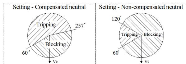
Fig. 8. Calibration of a directional protection.
