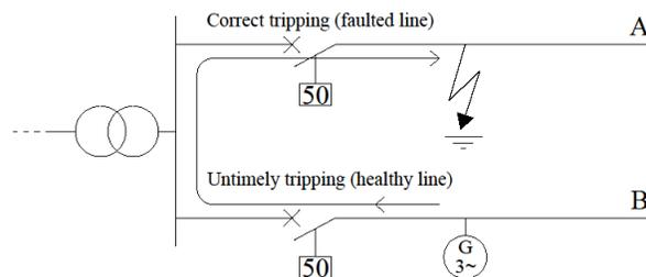
Fig. 12. Example of untimely tripping in a primary substation due to the massive presence of DG along the lines.
