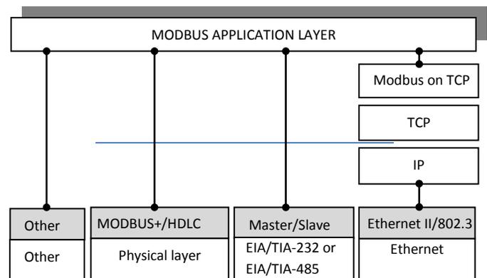
Fig. 11. Modbus communication stack.
