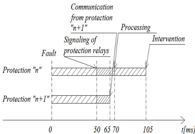
Fig. 6. Intervening times for the proposed logic.
