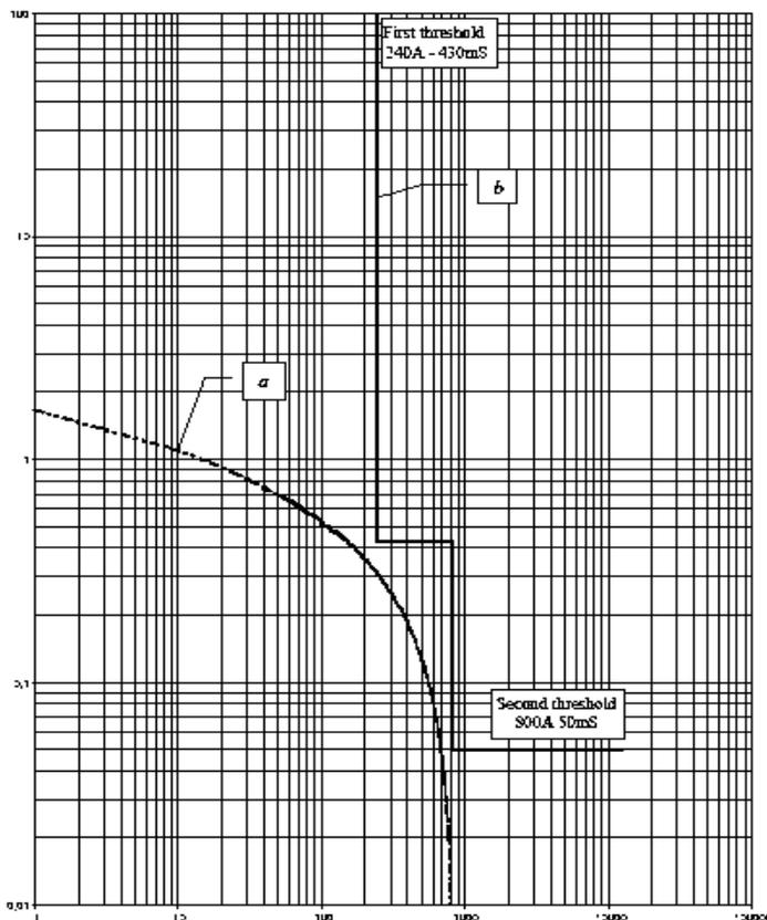
Fig. 10. Comparison of the characteristics of the transformer inrush current (a) and the circuit-breaker intervention (b).
