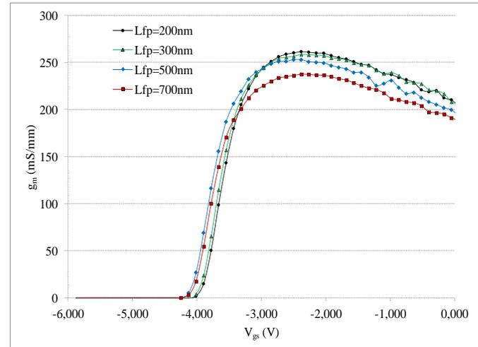
Fig. 6 Transconductance ( $g_m-V_{gs}$ ) characteristics of a  $0.6 \mu\text{m} \times 2 \times 100 \mu\text{m}$  AlGaIn/GaN HEMT with  $L_{fp} = 0.2, 0.3, 0.5,$  and  $0.7 \mu\text{m}$
