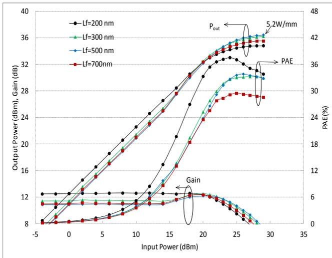
Fig. 8 Large-signal performance of the  $0.6 \mu\text{m} \times 6 \times 125 \mu\text{m}$  with  $L_{fp} = 0.2, 0.3, 0.5,$  and  $0.7 \mu\text{m}$  at 8 GHz. The device was biased with  $V_{ds} = 35 \text{ V}$  and  $V_{gs} = -2.4 \text{ V}$
