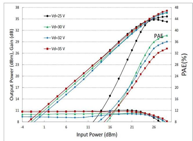
Fig. 10 Power performance versus drain bias  $V_{DS}$  for  $0.6 \mu\text{m} \times 8 \times 125 \mu\text{m}$  with  $L_{fp} 0.5 \mu\text{m}$  when measured at 8 GHz
