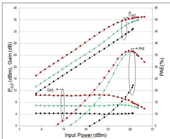
Fig. 11 Large-signal performance of the 0.6  $\mu\text{m}$   $\times$  8  $\times$  125  $\mu\text{m}$  with  $L_{fp} = 0.5 \mu\text{m}$  at 8 GHz, 10 GHz and 12 GHz. The device was biased with  $V_{ds} = 30 \text{ V}$  and  $V_{gs} = -2.4 \text{ V}$
