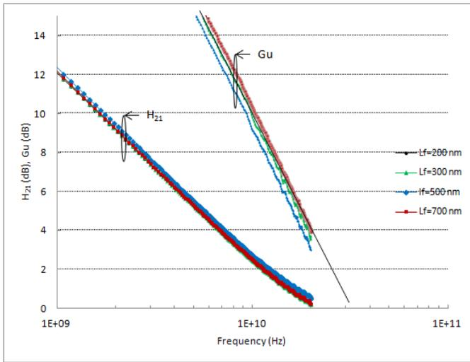
Fig. 7 Short-circuit current gain  $|h_{21}|$  and unilateral power gain of a  $0.6 \mu\text{m} \times 6 \times 125 \mu\text{m}$  AlGaIn/GaN HEMT with  $L_{fp} = 0.2, 0.3, 0.5,$  and  $0.7 \mu\text{m}$ . Device was biased at  $V_{DS} = 25 \text{ V}$  and  $V_{gs} = -3.0 \text{ V}$
