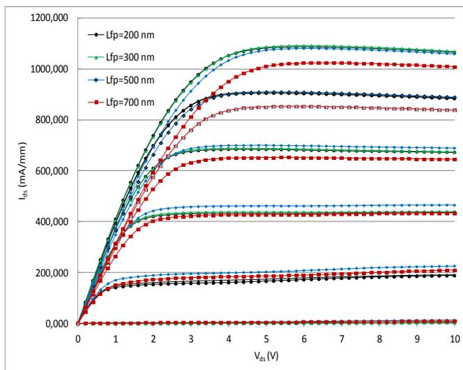
Fig. 5 Drain current-voltage ( $I_{DS}-V_{DS}$ ) characteristics of a  $0.6 \mu\text{m} \times 2 \times 100 \mu\text{m}$  AlGaIn/GaN HEMT with  $L_{fp} = 0.2, 0.3, 0.5,$  and  $0.7 \mu\text{m}$ . The gate bias was swept from  $-4$  to  $1 \text{ V}$  in a step of  $1 \text{ V}$
