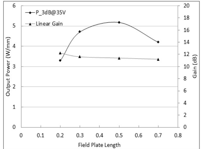
Fig. 9 Power performance versus length of field plate  $L_{fp}$  for devices of  $0.6 \mu\text{m} \times 6 \times 125 \mu\text{m}$  when measured at 8 GHz with drain biases of 35 V
