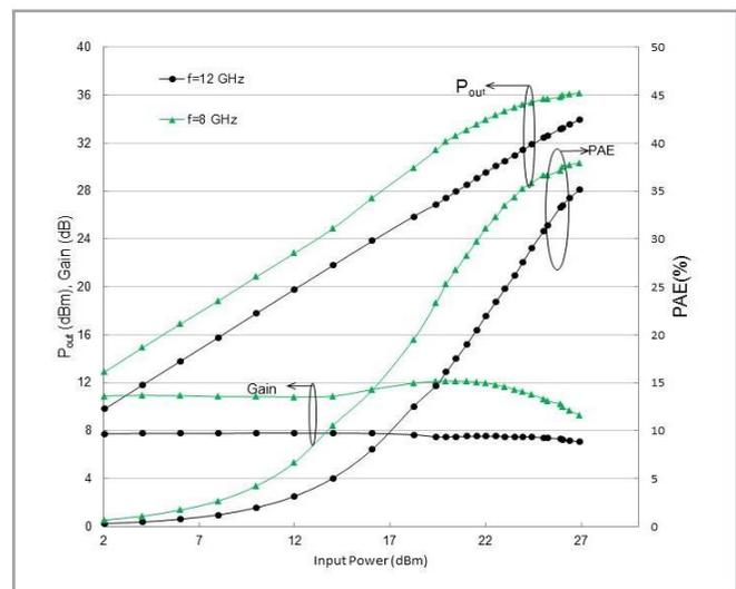
Fig. 12 Large-signal performance of the 0.6  $\mu\text{m}$   $\times$  6  $\times$  125  $\mu\text{m}$  with  $L_{fp} = 0.5 \mu\text{m}$  at 8 GHz and 12 GHz. The device was biased with  $V_{ds} = 30 \text{ V}$  and  $V_{gs} = -2.4 \text{ V}$
