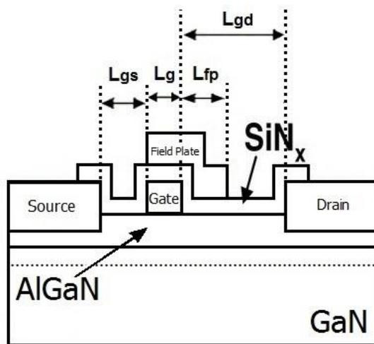
Fig. 2 Schematic of field-plated AlGaIn/GaN HEMT structure
