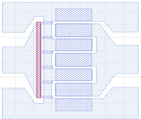
Fig. 1 Layout of the field-plated AlGaIn/GaN HEMT structure
