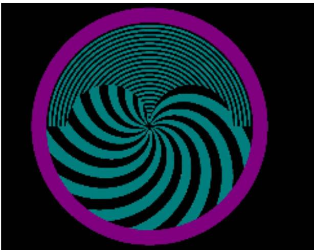
Figure 3: Negative image of the modulator disk
