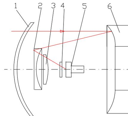
Figure 1: Optical scheme of the coordinator
