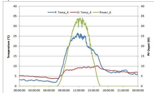
Fig. 9 PV surface temperature, outside temperature and PV output power comparison for Kırklareli
