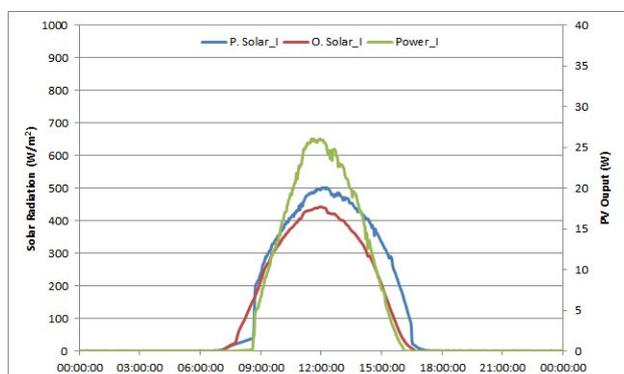
Fig. 8 PV surface solar radiation, outside solar radiation and PV output power comparison for İstanbul
