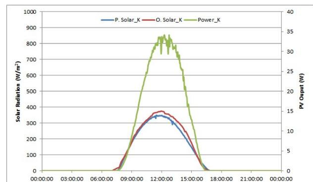
Fig. 10 PV surface solar radiation, outside solar radiation and PV output power comparison for Kırklareli
