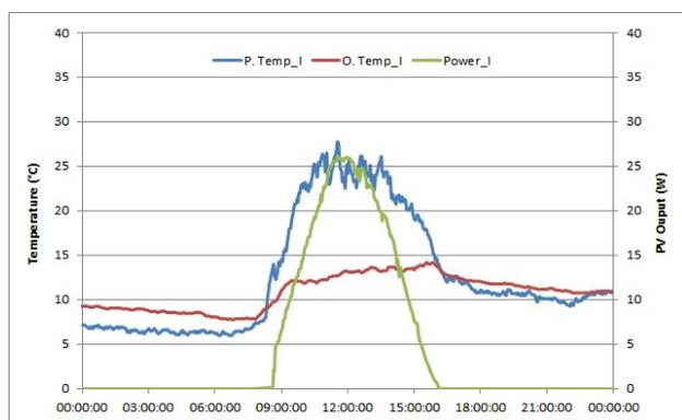
Fig. 7 PV surface temperature, outside temperature and PV output power comparison for İstanbul
