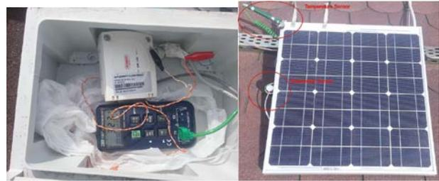
Fig. 5 Thermometer and solarimeter with their probes mounted on PV panel.
