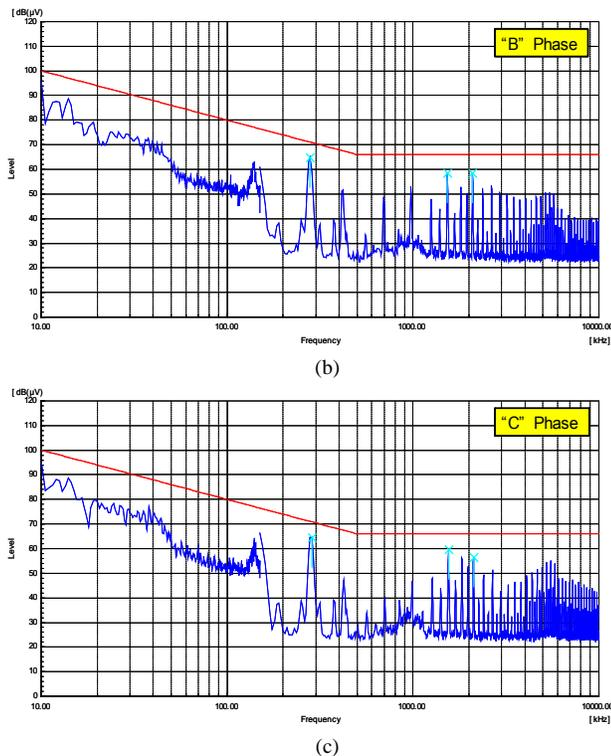
Fig. 12 Measuring the power supply noise after the filter application, (a) Conducted noise of A phase, (b) Conducted noise of B phase, (c) Conducted noise of C phase
