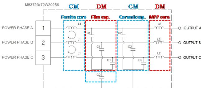
Fig. 6 Power filter circuit diagram
