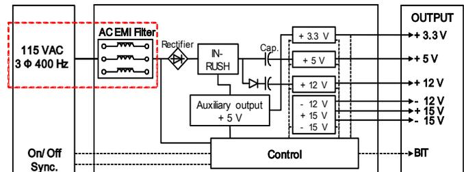
Fig. 11 Block diagram of the switch power supply with EMI filter
