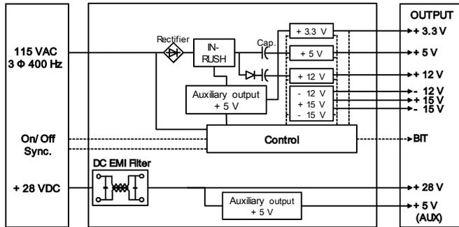
Fig. 2 switch power supply block diagram
