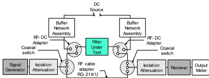
Fig. 9 MIL-STD-220B : Concept for measuring the attenuation characteristics of the filter
