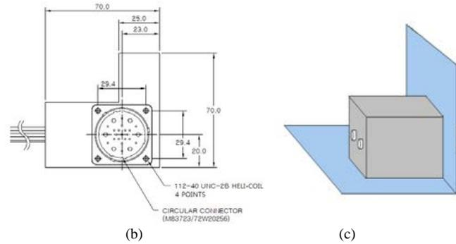
Fig. 7 Shape and dimensions, (a) Side view, (b) Top view, (c) Integrated structure
