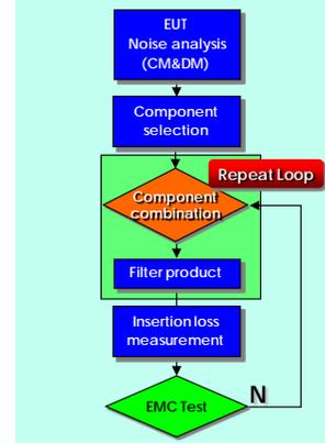
Fig. 5 Power filter design flow diagram
