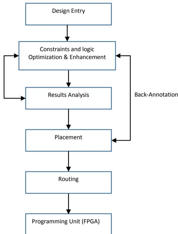
Fig.1 Design Flow Process Diagram
