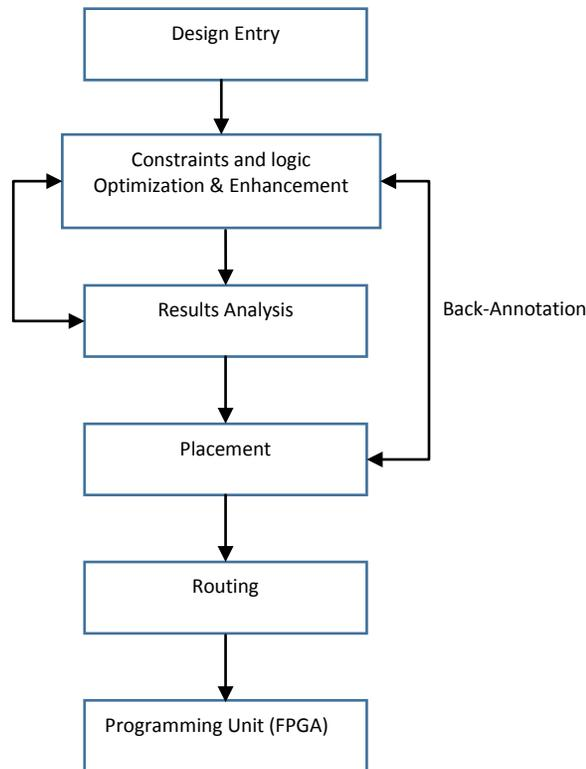
Fig.1 Design Flow Process Diagram
