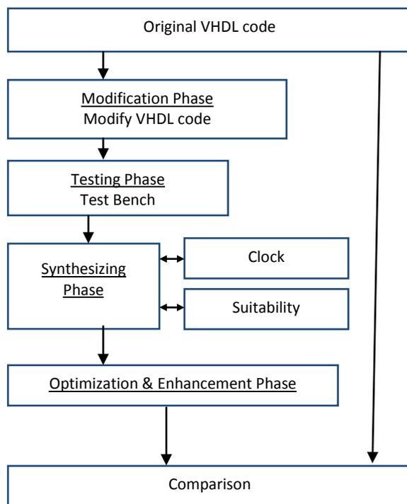
Fig. 2: Architecture of the Proposed Enhancement
