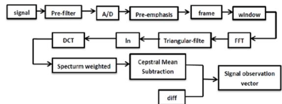
Fig. 4 The processing of MFCC extracts signal characteristics
