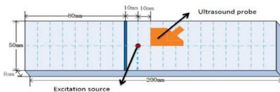
Fig. 1 The schematic diagram for the experiment of reflected wave measurement
