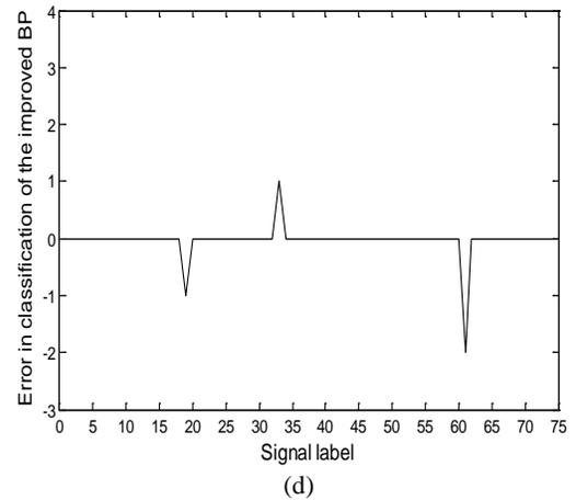
Fig. 6 Reflected wave experiment contrast. (a) BP network classification results of reflected wave. (b) Error of BP network classification. (c) The improved BP network classification results of reflected wave. (d) Error of the improved BP network classification.
