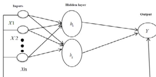
Fig.8 Feedforward neural network with jump connections
