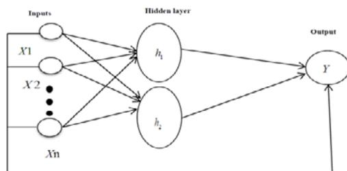
Fig.8 Feedforward neural network with jump connections
