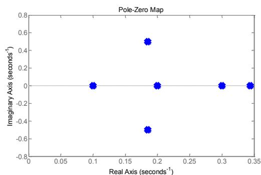
Fig. 18 Pole map of control nominal model  $G_{N_2}(z^{-1})$
