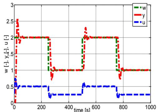
Fig. 15 Control of perturbed model  $G_{\Delta P2}(z^{-1})$  -  $K = 4$
