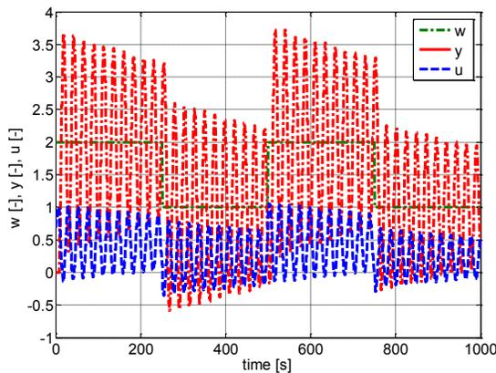
Fig. 7 Control of perturbed model  $G_{p3}(z^{-1})$ ,  $K = 4.4$
