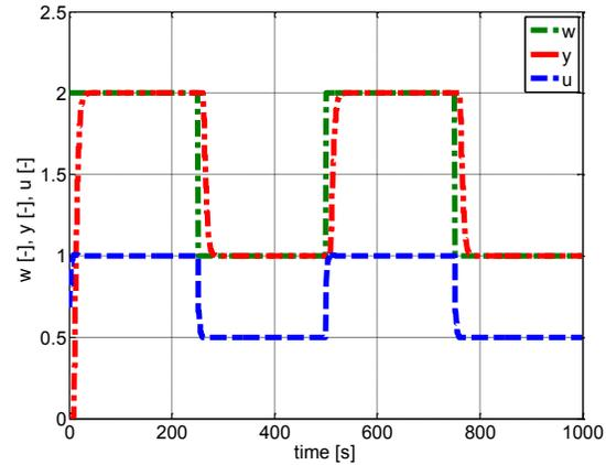
Fig. 3 Control of nominal model  $G_{N1}(z^{-1})$ ,  $K = 2$
