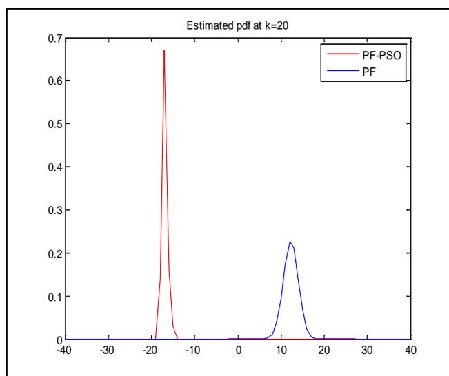
Fig. 2 The height and width of the pdf corresponding to the error attained by the PF-PSO filter reflect its better performance in comparison to the PF estimation techniques.
