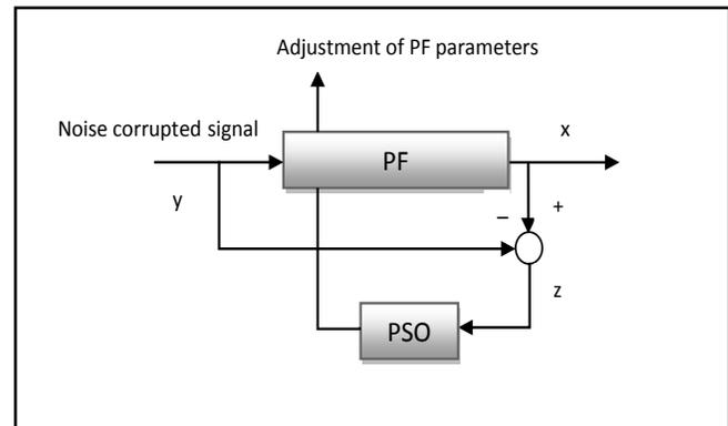
Fig. 2 PF-PSO functional block diagram.
