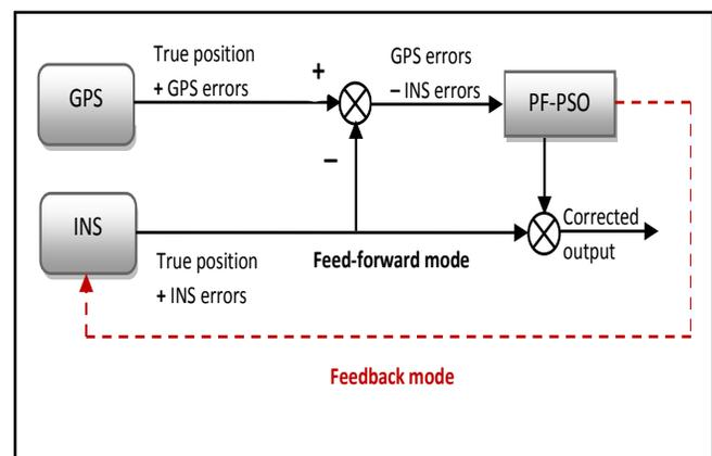
Fig. 3 Proposed approach in GPS/INS integration.
