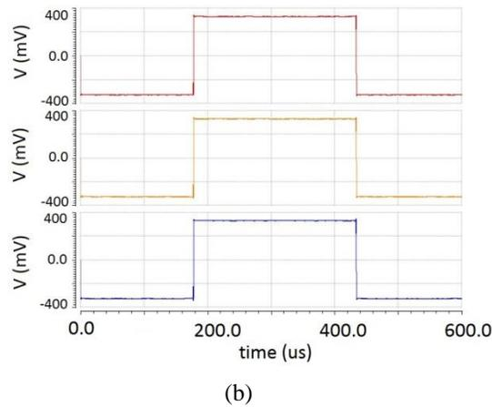
Fig. 10: Output signals of comparators – a) Pulses of phasing . b) Phased Square waves
