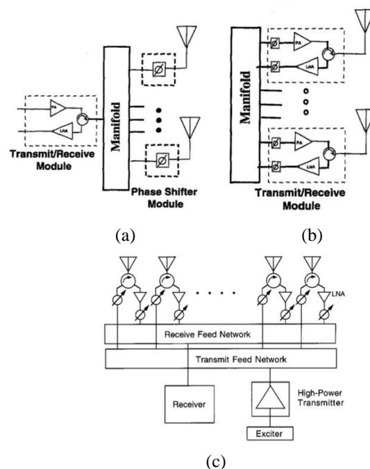
Fig. 1: Electronically Scanned Arrays (a) Passive ESA, (b) Active ESA, (c) Hybrid ESA.
