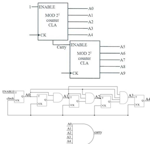
Fig. 6 Simplified 10-bits counter. (a) Parallel/Serial Connection. (b) Simplified schematic of the first 5-bits CLA counter.
