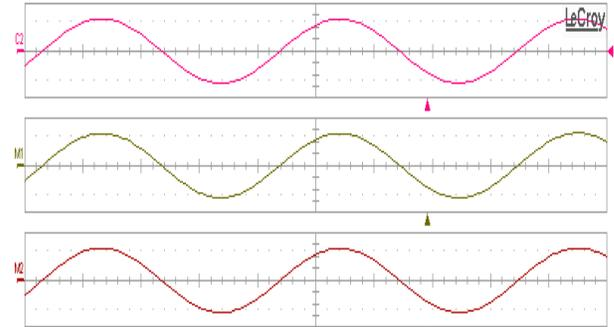
Fig. 18: VCO measured output waveforms with the same phase control word for all the three channels
