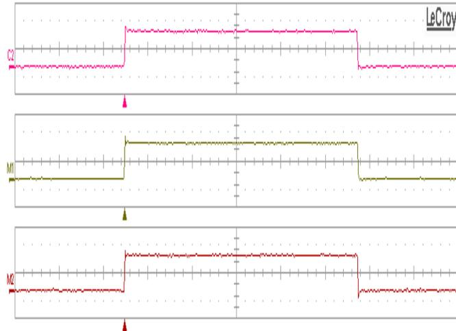
Fig. 13: PCB measured output waveforms with the same phase control word for all the three channel
