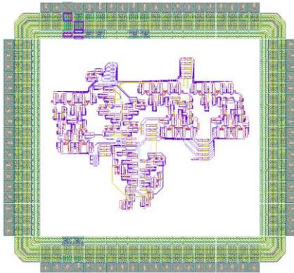
Fig. 4: Phase Shifter – Final Layout
