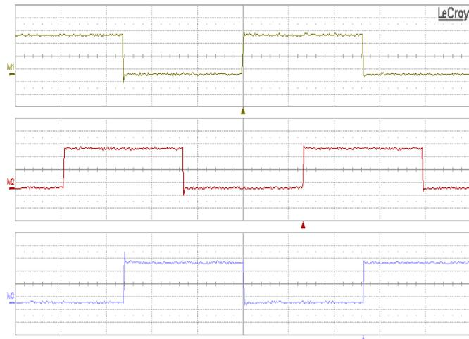
Fig. 14: PCB measured output squared waves with 90° and 180° phase shift.
