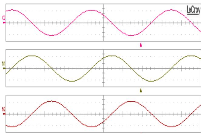
Fig. 22: VCO measured output waveforms with  $90^\circ$  and  $180^\circ$  phase shift
