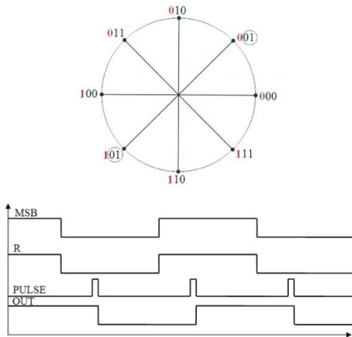
Fig. 8: Principle of comparators operation.
