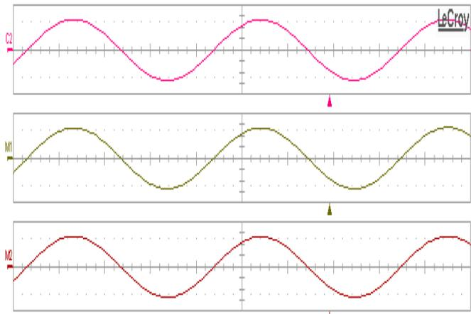
Fig. 21: VCO measured output waveforms with the same phase control word for all the three channels
