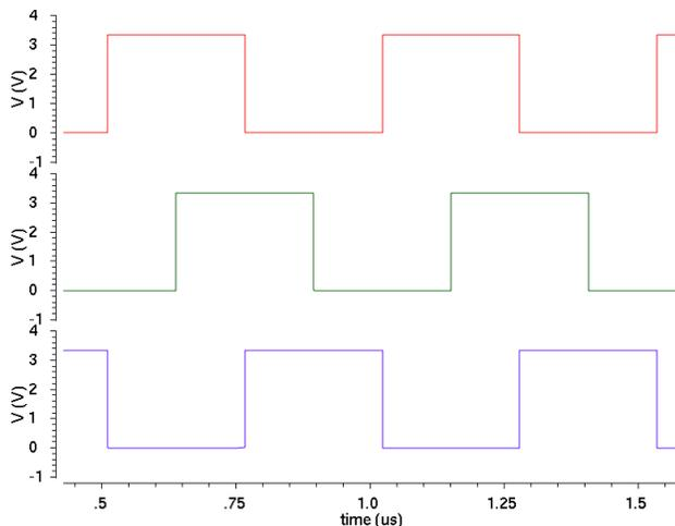
Fig. 11: PCB simulated output squared waves with  $90^\circ$  and  $180^\circ$  phase shift .
