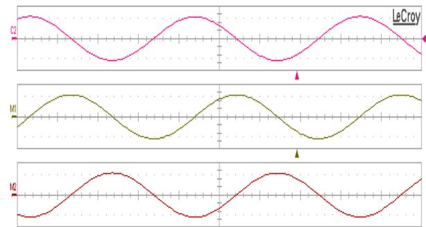
Fig. 19: VCO measured output waveforms with 90° and 180° phase shift
