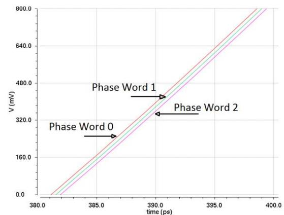
Fig. 12:  $2.4 \text{ GHz}$  phased output signal
