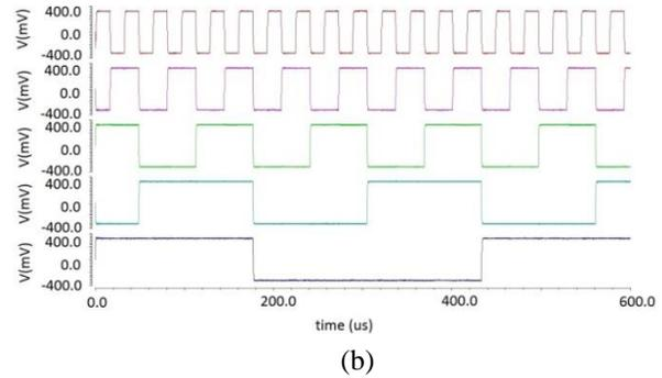
Fig. 9 10-bit Counter Outputs: (a) LSB bits (b) MSB bits
