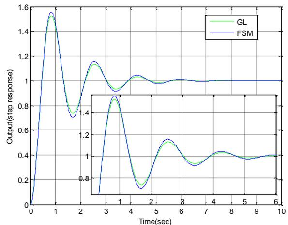
Fig. 7: Step responses obtained from GL method and FSM.
