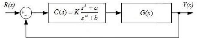
Fig. 2: A closed loop control system with fractional order controller
