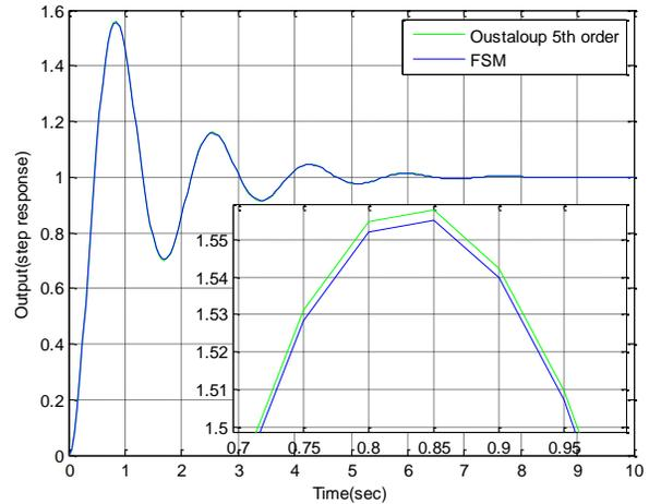
Fig. 6: Step response of the system obtained from FSM and the step responses of  $P_{ous5}(s)$
