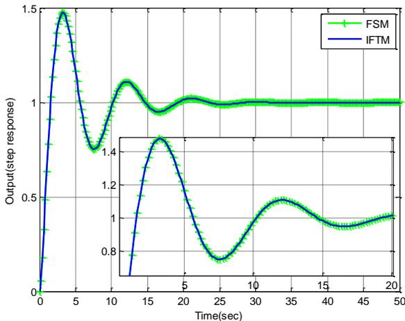
Fig. 8: Step responses obtained from FSM and IFTM.
