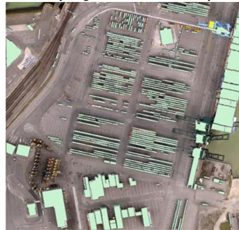
Fig. 9 Overlay of extracted building roofs over color orthophoto.
