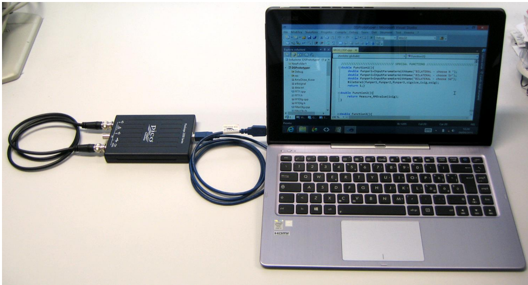
Fig.2 – Development environment running on a notebook interfaced to a multi-function oscilloscope. (The output of the signal generator is connected to the input channel A).
