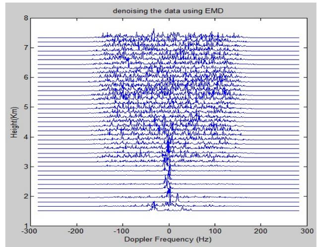
Fig. 9 After denoising the original data using EMD
