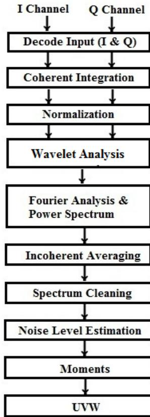
Fig. 3 Data processing steps of LAWP Radar
