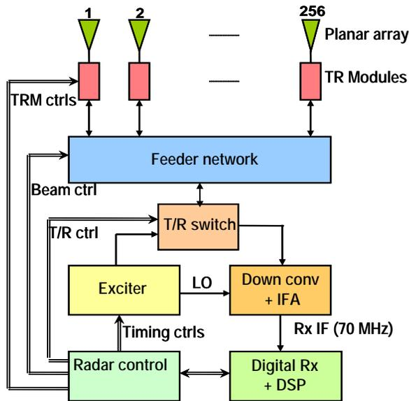
Fig. 1 Block diagram of LAMP Radar
