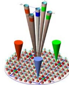
Fig. 2 Antenna Configuration for Doppler Beam Swinging Technique
