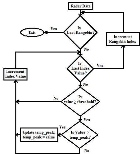
Fig. 4 Flow diagram of the Peak Detection Technique
