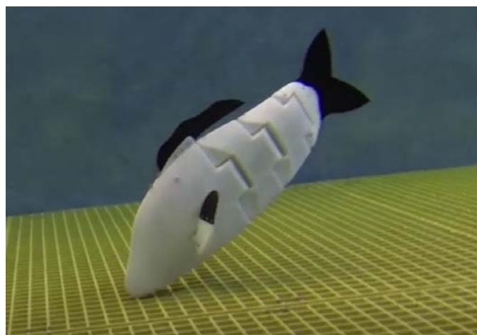
Fig. 1. BUV CyberFish ver. 5 in a swimming pool [6]
