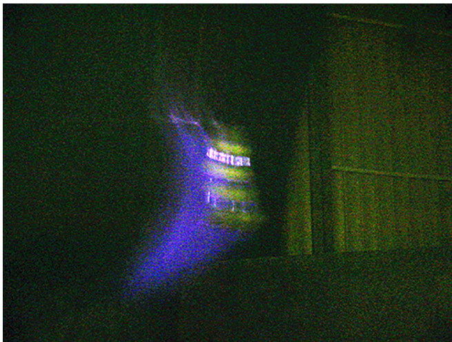
Fig. 7. Powerful streamer discharges initiated by the model hydrometeor array between the positive and negatively charged artificial thunderstorm cells
