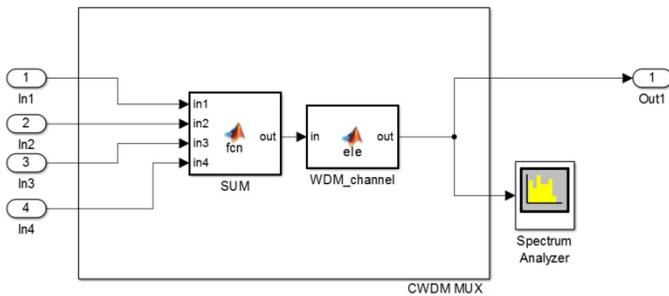
Fig. 7 The principle scheme of the CWDM MUX block
