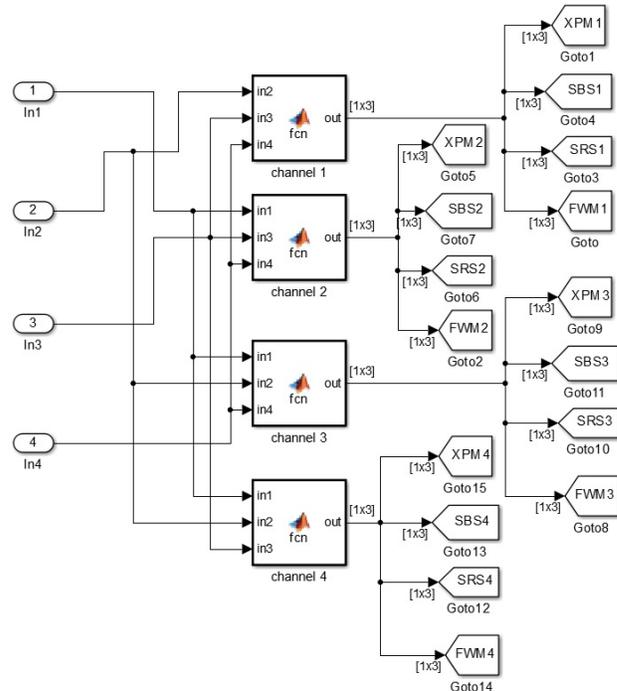
Fig. 10 The detailed scheme with internal connection of the Nonlinear effects block for the 4-channel CWDM system
