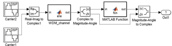
Fig. 5 The functional scheme of the CW signal source
