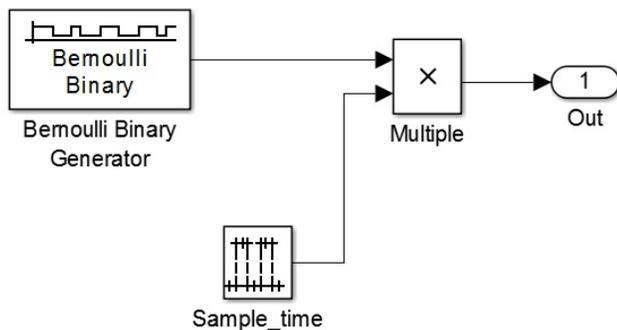
Fig. 4 The functional scheme of the Data signal source
