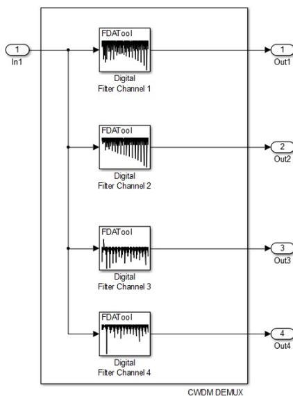
Fig. 8 The detailed scheme with internal connections of the CWDM DEMUX block
