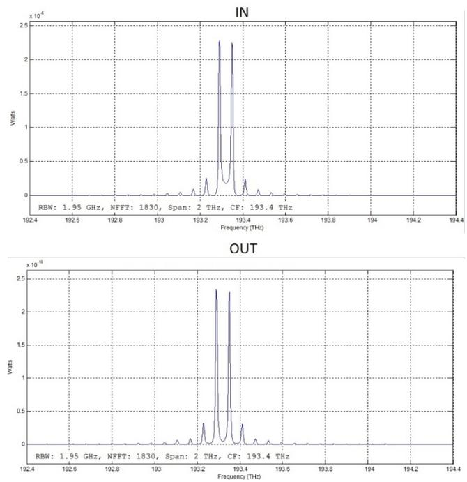
Fig. 12 The detailed frequency spectrum of the 2. CWDM channel (a) entering IN and (b) outgoing OUT the SMF block
