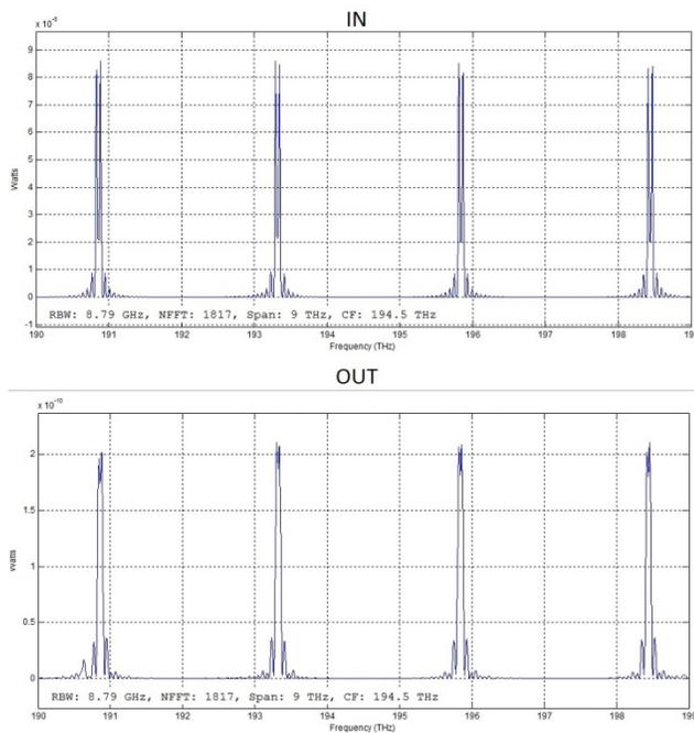
Fig. 11 The frequency spectrum of four CWDM channels (a) entering IN and (b) outgoing OUT the SMF block
