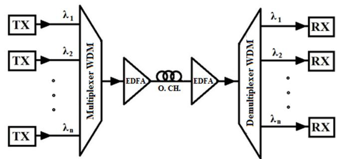
Fig. 2 The principle scheme of the WDM system
