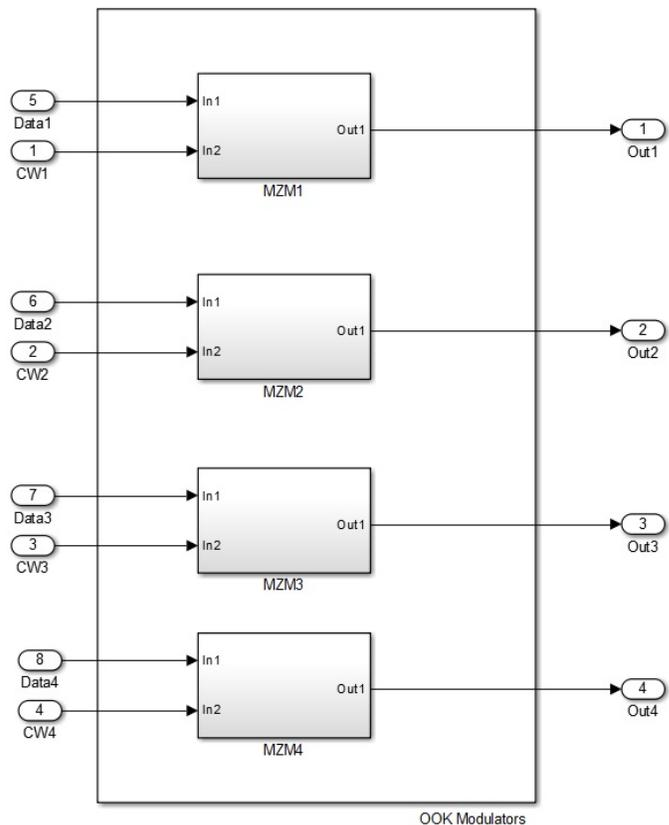
Fig. 6 The detailed scheme with internal connections of the OOK Modulators block
