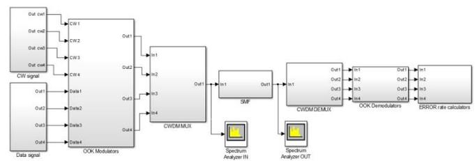
Fig. 3 The Simulink model of the 4-channel CWDM optical transmission path
