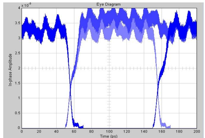
Fig. 9 The eye diagram for OOK optical signals after transmitting in the 80 km optical transmission path using the 4-channel CWDM system
