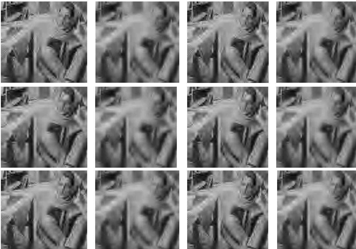
Fig. 5. Results of SureShrink thresholding method for denoising Barbara by using Median absolute deviation (first row), Quantile median (second row), Marginal variance (third row) for noise power estimation and Hard (first column), Soft (second column), Exp. (third column), Garrot (forth column) as the thresholding rule under noise variance 0.3.
