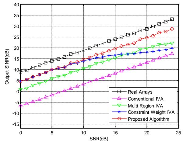
Fig.6 Analysis output SINR under large transformation angle
