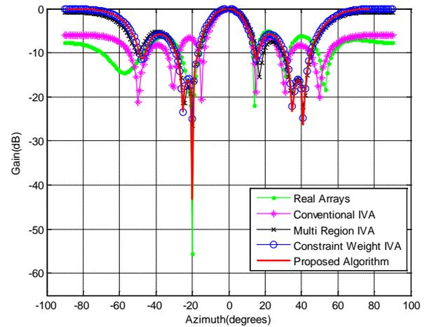
Fig.5 Analysis beamforming under large transformation angle
