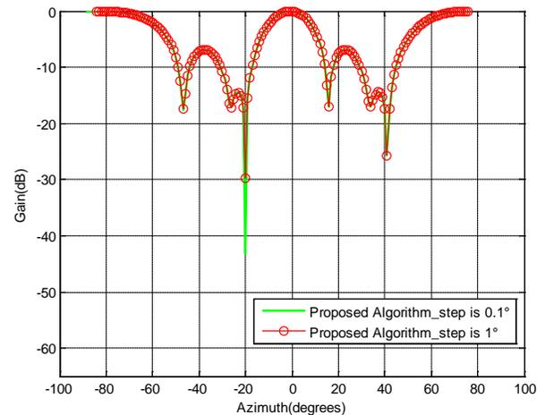
Fig.9 Analysis accuracy with different interpolation step
