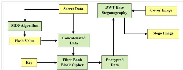
Fig. 2 Transmitter Block Diagram
