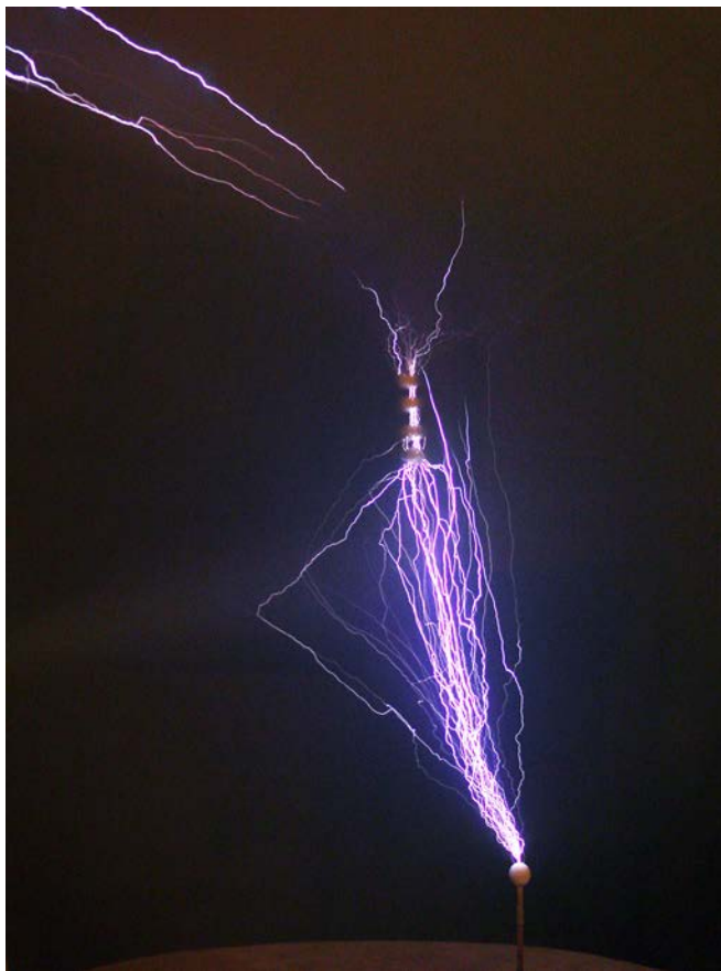
Fig. 15. Powerful channel discharges initiated by the model hydrometeor arrays in the system of the negatively charged artificial thunderstorm cells and between the cells and the grounded parts of the aerosol chamber
