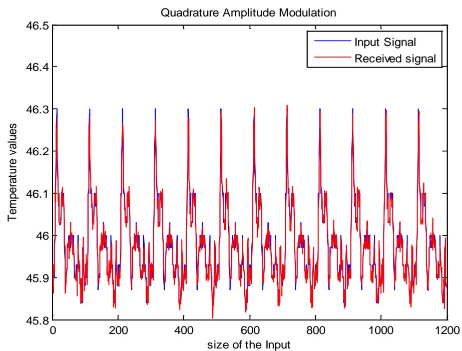
Fig.3 Input and Reconstructed (received) signal with differential encoding and QAM modulation
