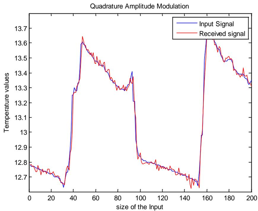
Fig.5 Input and Reconstructed (received) signal with differential encoding and QAM modulation
