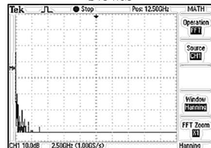
(d) Waveform of current harmonic distribution using the proposed random zero vector SVPWM
