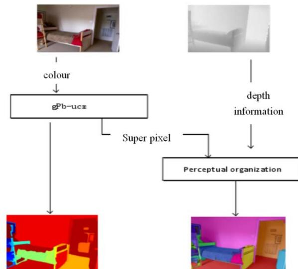
Fig. 3. Segmentation algorithm framework based on RGB-D indoor scene
