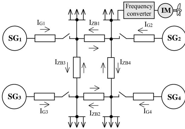
Fig. 1. Scheme of investigated ship's power system
