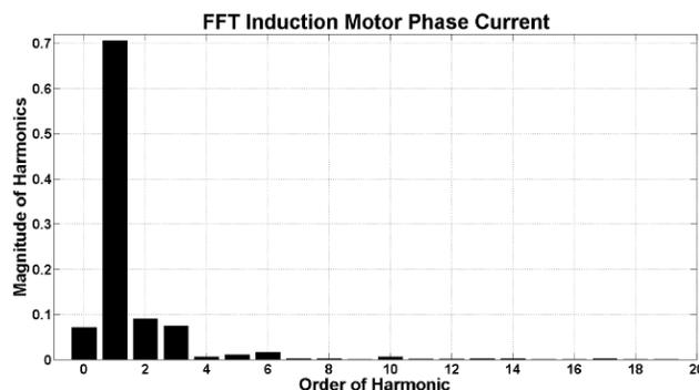
Fig.19. Harmonic of motor phase current
