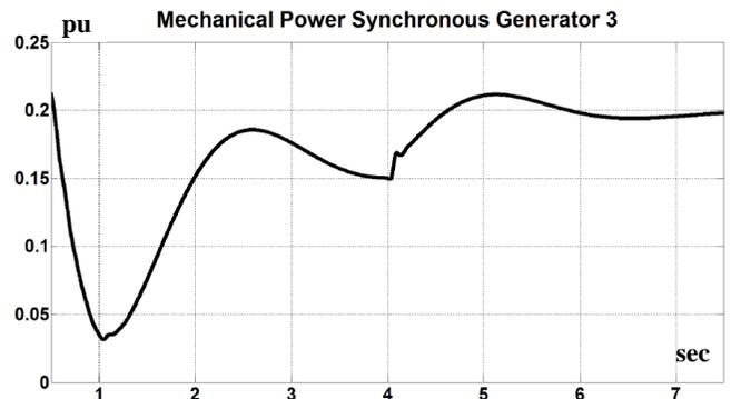
Fig.15. Synchronous generator #3 mechanical power
