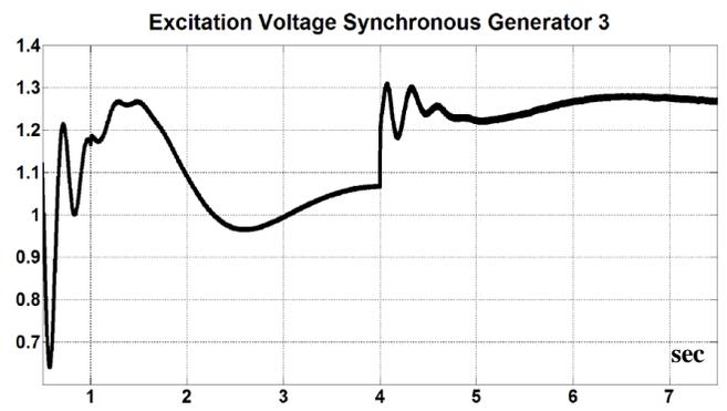
Fig.16. Excitation voltage of generator #3
