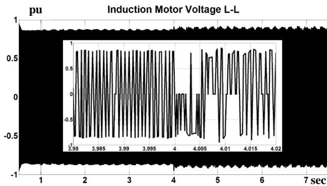
Fig.11. Induction motor line-to-line voltage
