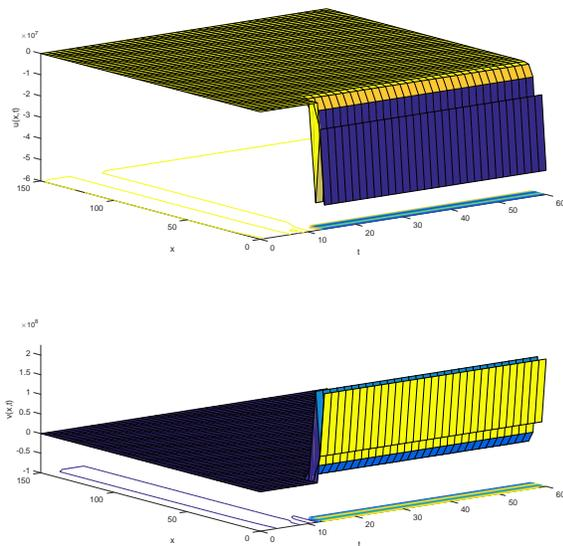
Fig. 2. Numerical solution of  $\lambda - \omega$  reaction-diffusion system (I.1), with initial conditions (II.4) and boundary conditions (II.7) computed by a standard IMEX method with spatial stepsize  $h = 3$  and time stepsize  $k = 1.5$ . The component  $u(x, t)$  is depicted on the top and the component  $v(x, t)$  is represented on the bottom.
