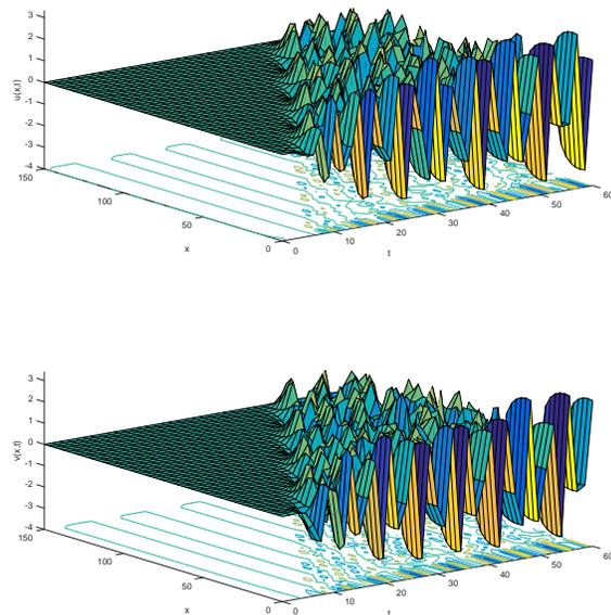
Fig. 3. Numerical solution of  $\lambda - \omega$  reaction-diffusion system (I.1), with initial conditions (II.4) and boundary conditions (II.7) computed by the new method (III.18) with spatial stepsize  $h = 3$  and time stepsize  $k = 1.5$ . The component  $u(x, t)$  is depicted on the top and the component  $v(x, t)$  is represented on the bottom.
