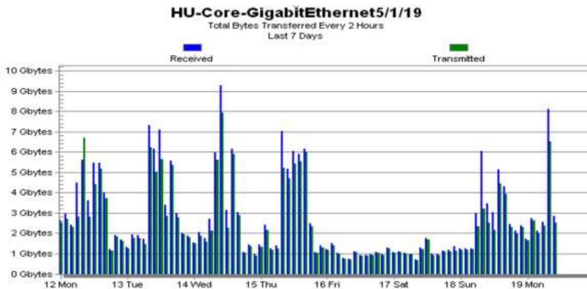
Fig. 8 The transmit (upload) over main core interface where proxy server connected and the receives (download) packets
