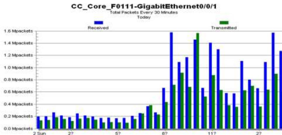
Fig.5 The received (upload) over the main interface compared to transmitted (download) packets
