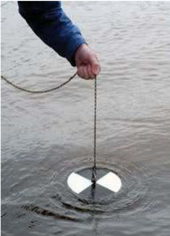
Fig.3 Depth and turbidity measurement using Secchi disc
