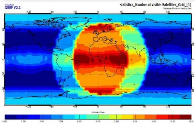
Fig. 9. Visibility of GPS and SBAS systems satellites
