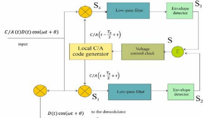
Fig. 2. A loop tracking the phase of the C/A code with a fixed delay [12]
