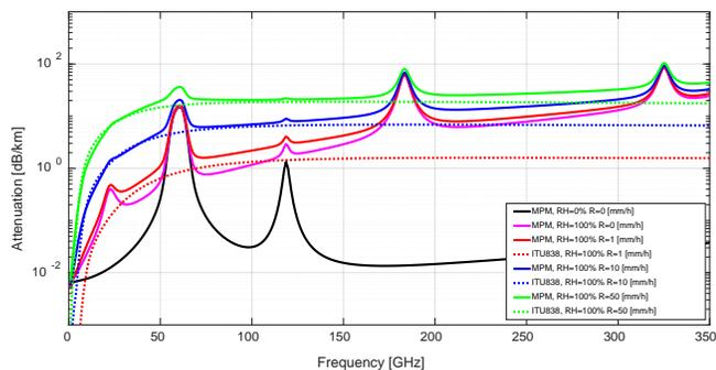
Fig. 5: Comparison of MPM and ITU-P.838 recommendation for different relative humidity  $RH$  [%] and rainfall rate  $R$  [mm/h].
