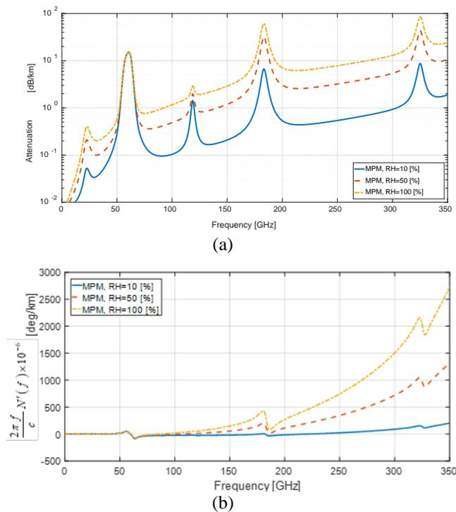
Fig. 1: (a) Attenuation and (b) incremental phase dispersion propagation factors in different conditions of relative humidity RH [%]
