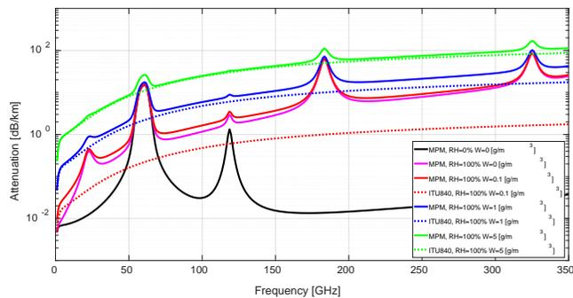
Fig. 4: Comparison of MPM and ITU-P.840 recommendation for different relative humidity  $RH$  [%] and liquid water content  $W$  [g/m<sup>3</sup>]
