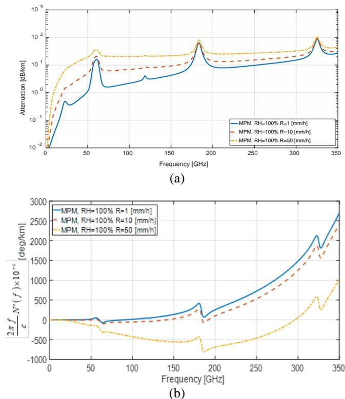
Fig. 3: (a) Attenuation and (b) incremental phase dispersion propagation factors in different conditions of rainfall rate  $R$  [mm/h]
