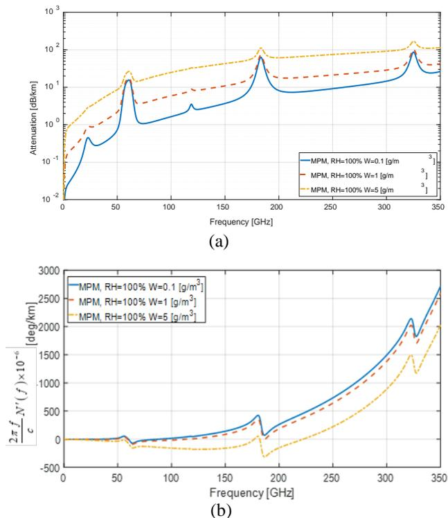
Fig. 2: (a) Attenuation and (b) incremental phase dispersion propagation factors in different conditions of liquid water content W [g/m<sup>3</sup>]
