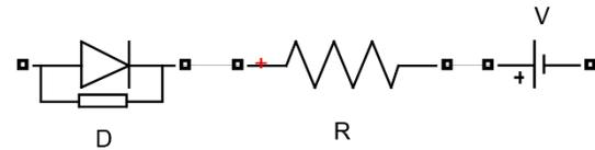
Fig. 2. Electrical modeling of LED in MATLAB Simulink
