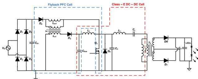
Fig. 2.3. Circuit of LED driver based on Flyback and Class – E converter [24]
