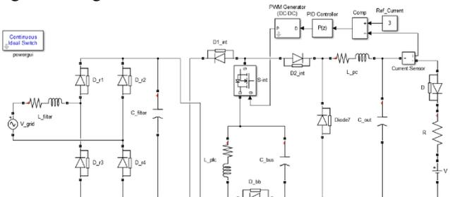
Fig. 1. Circuit diagram of integrated DC-DC converters [17].
