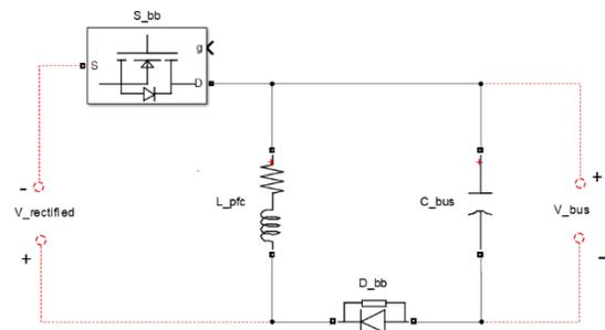
Fig. 3. Buck-boost converter
