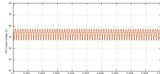
Fig. 6. Ripple in PFC output voltage.
