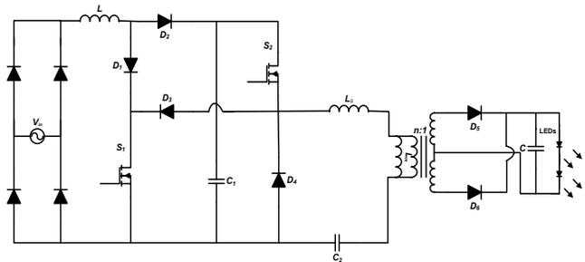
Fig. 2.1. Circuit of LED driver based on Boost circuit and LLC converter [21]
