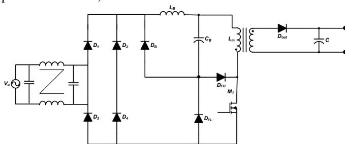
Fig. 2.2. Circuit of Integrated Buck Flyback LED driver with EMI Filter [18]
