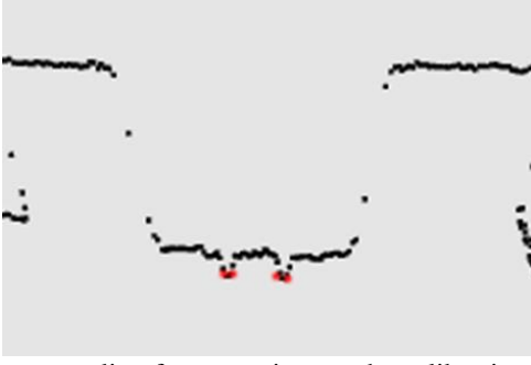
Fig.9 Corresponding feature points on the calibration board in the 2D point cloud
