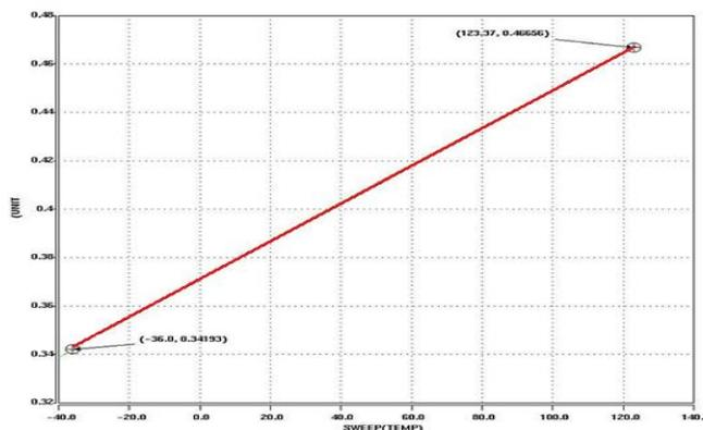
Fig. 4 Simulation results of the variation of the Ron with temperature variation
