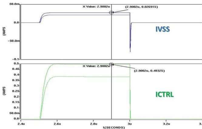
Fig. 11. Simulation results of the current IVSS & ICTRL in transient mode
