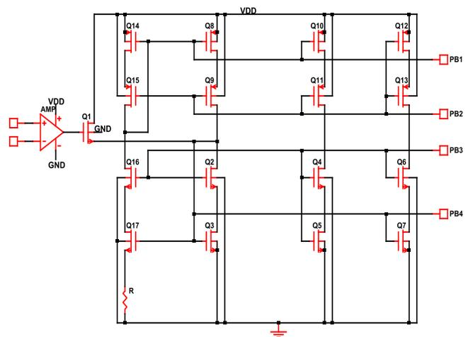
Fig. 12 PMOS Bias Voltage architecture
