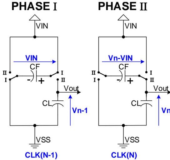
Fig. 1 Block diagram of the operation of the charge pump voltage doubler
