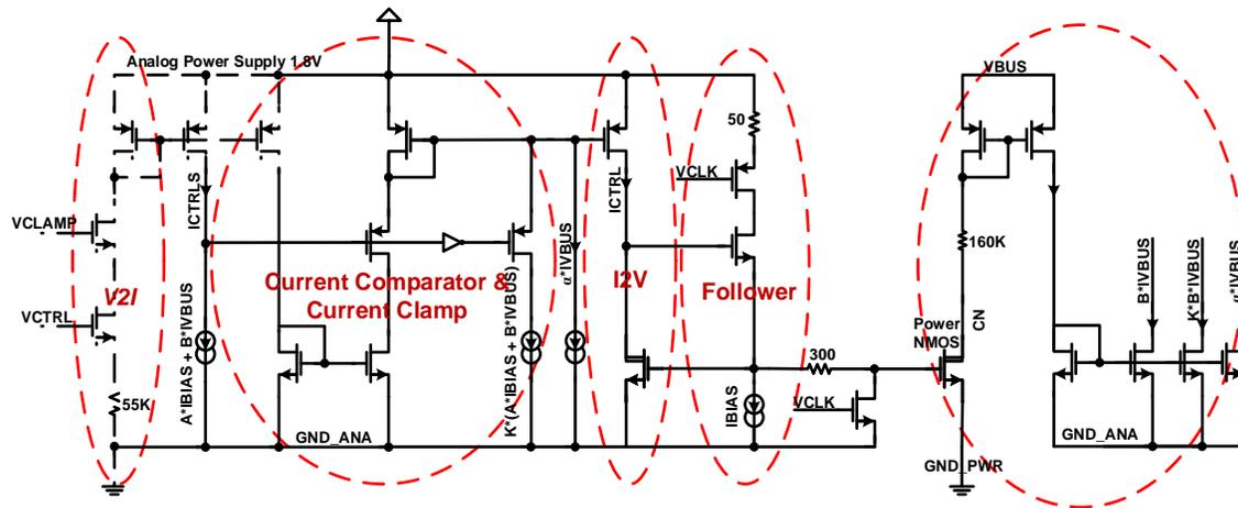
Fig. 10 Current mode control architecture
