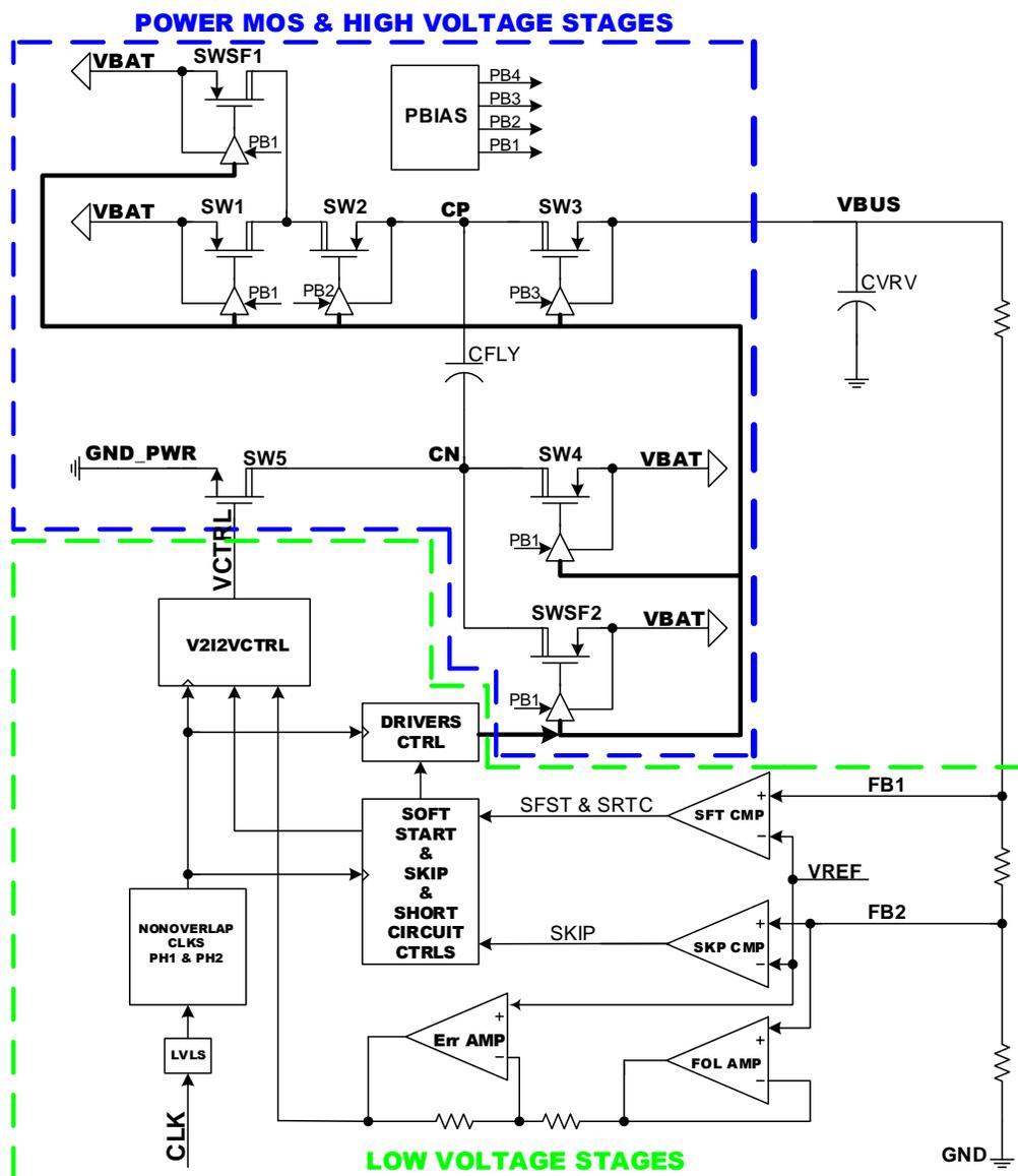
Fig. 3 The proposed charge pump block diagram
