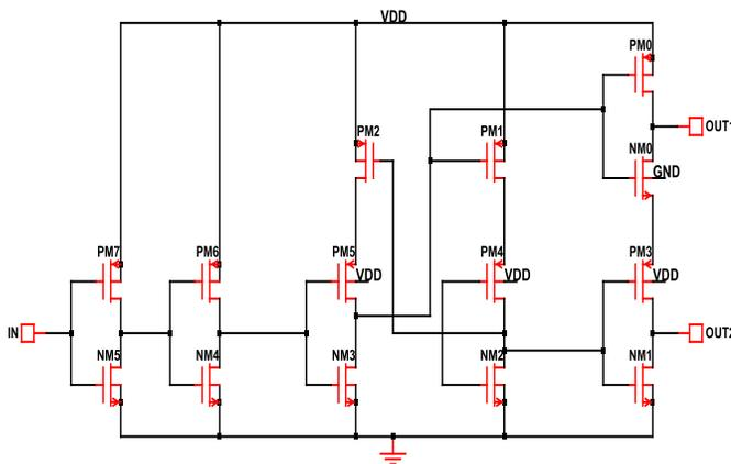
Fig. 6 Circuit design of the Low Voltage Level Shifter
