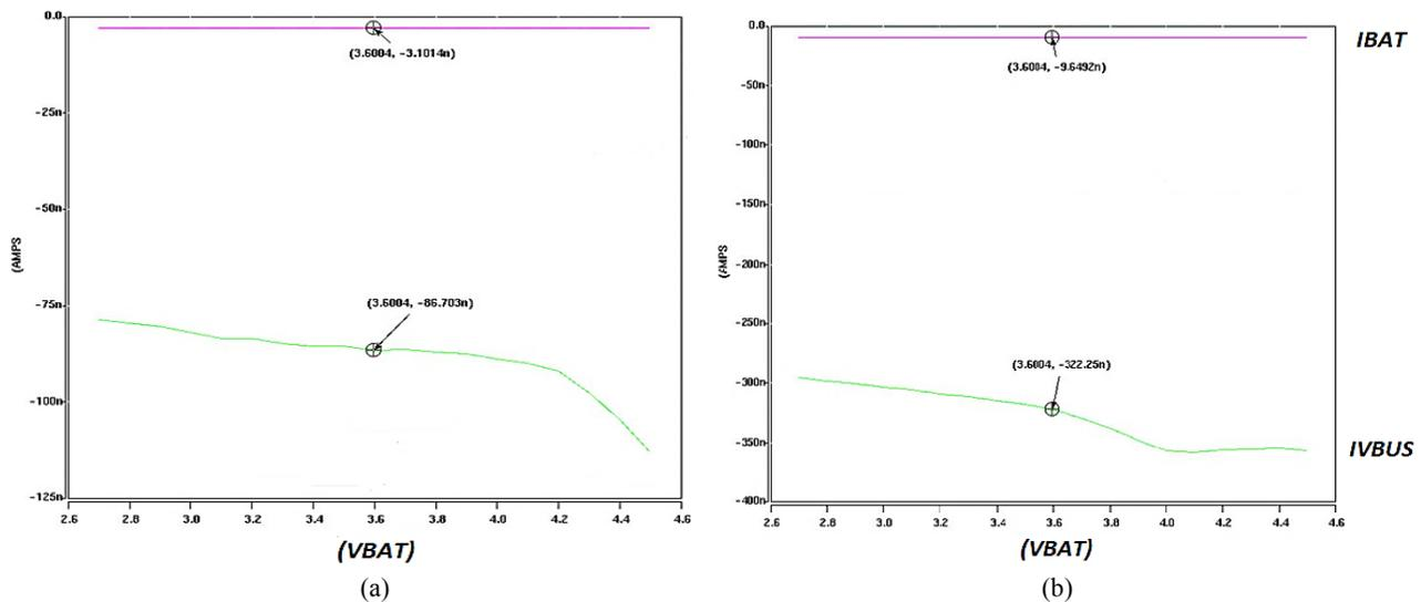
Fig. 15. Simulation results of nominal voltage leakage for IBAT and IVBUS in: (a) Nominal Process, and (b) Strong Process
