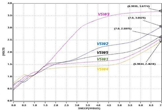
Fig. 5 Simulation results of the variation of the (SW1, SW2, SW3, SW4, SW5) voltages with VBUS varying from 0 to 7V
