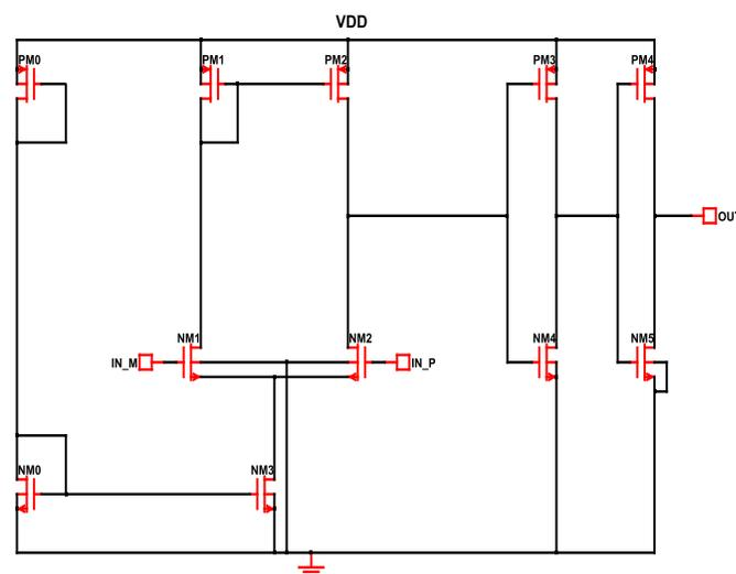
Fig. 9 Circuit design of the comparator used in soft start mode and skip mode
