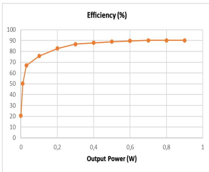
Fig. 17 System efficiency versus output power with  $f_{in}=1\text{MHz}$
