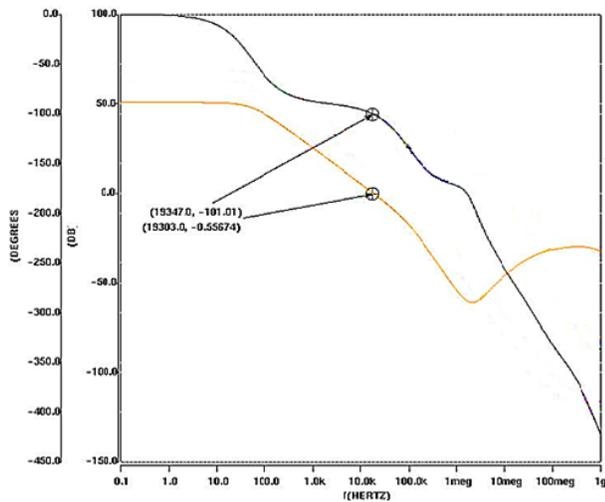
Fig. 16 Stability simulation result
