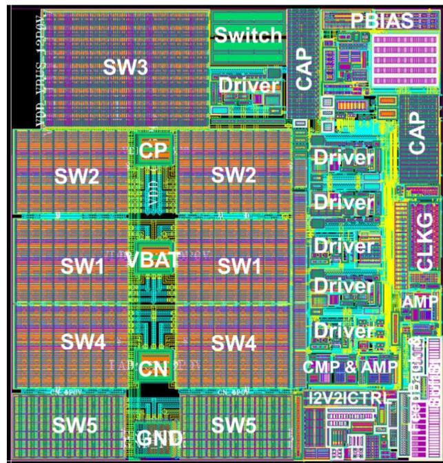
Fig. 18 Layout of the proposed charge pump
