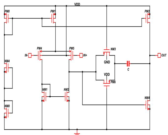
Fig. 7. Circuit design of the amplifier used as error amplifier and follower amplifier
