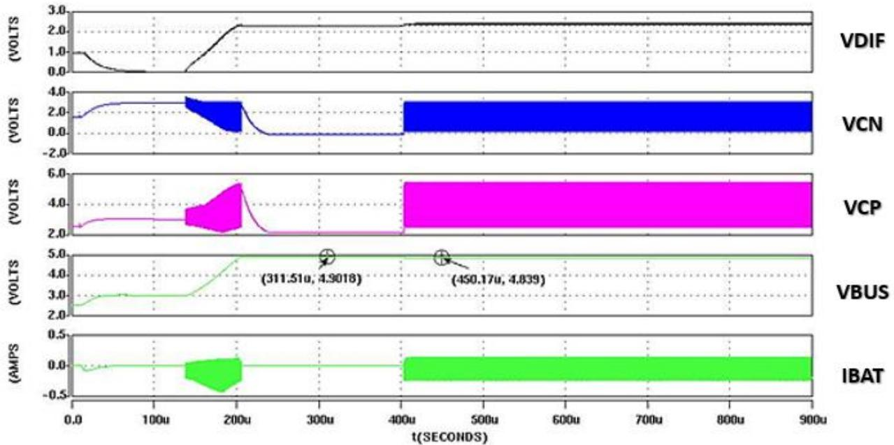
Fig. 14 Simulation results of the functionality of the proposed charge pump
