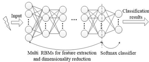
Fig. 1 basic principle of DBN fault classification
