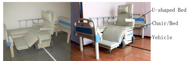
Fig. 18. The overview of the chair-bed system
