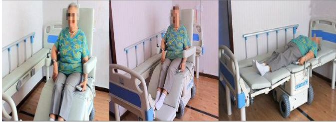
Fig. 1. The docking process of the system
