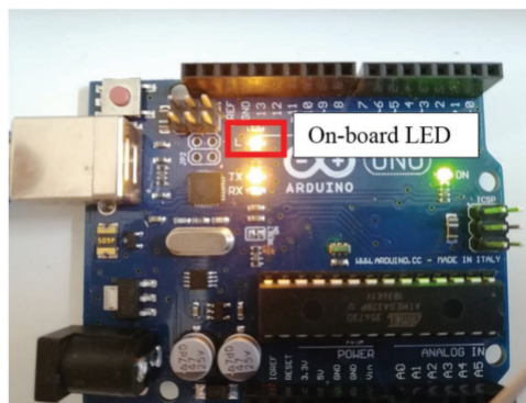
Fig. 19: The on-board LED will be switched on when the muscle contracts.
