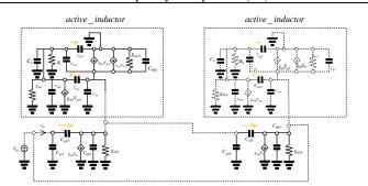
Figure 4. The high frequency equivalent circuit of the commonsource cross-coupled amplifier with NMOS only active inductor.
