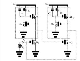
Figure 1. The Circuit diagram of "The common-source cross-coupled amplifier with NMOS only active inductor"
