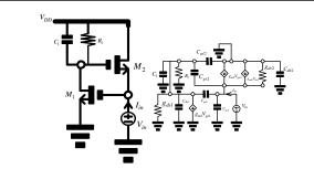
Figure 2. The input impedance of the NMOS only active inductor and its high frequency equivalent circuit of the first stage resonance circuit
